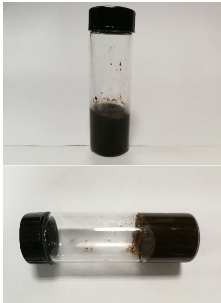
Figure S2. Photograph images of the \text{NH}_2\text{-MIL-101(Fe)@GO} hydrogel.
