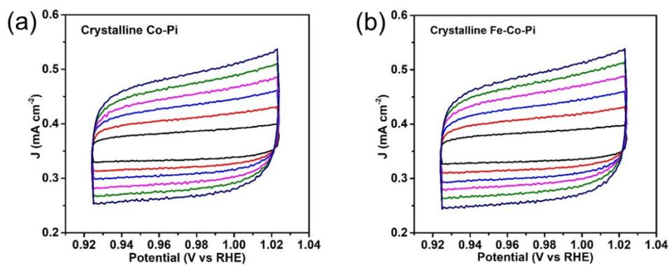
**Fig. S13** Cyclic voltammograms of (a) crystalline Co-Pi and (b) crystalline Fe-Co-Pi with a potential window from 0.924 to 1.024 V at different scan rates in 1.0 M KOH.
