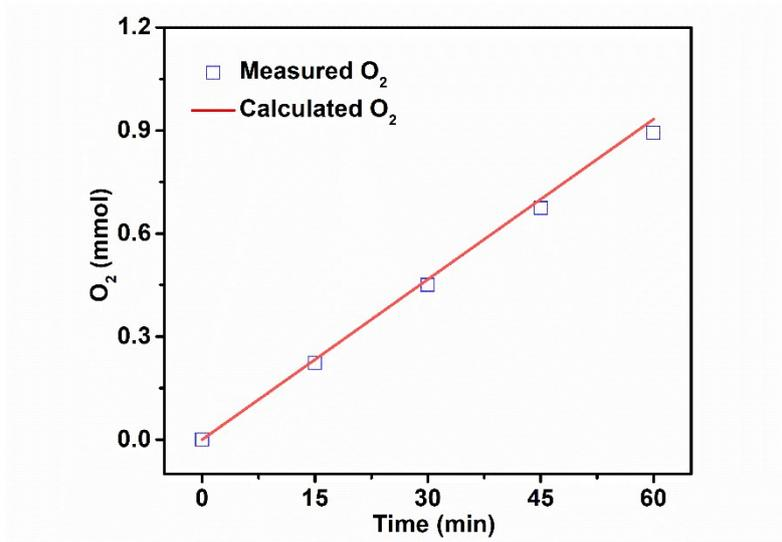
**Fig. S6** The amount of theoretically calculated and experimentally measured oxygen as a function of time for Am Fe-Co<sub>3</sub>(PO<sub>4</sub>)<sub>2</sub> at a constant current density of 100 mA cm<sup>-2</sup>.
