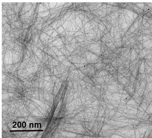
**Fig. S7** TEM image of Am Fe-Co<sub>3</sub>(PO<sub>4</sub>)<sub>2</sub> ultrathin nanowires after stability test for the OER.
