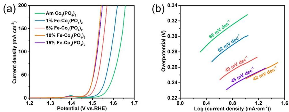
**Fig. S10** (a) LSV curves of Am Co<sub>3</sub>(PO<sub>4</sub>)<sub>2</sub> and Am Fe-Co<sub>3</sub>(PO<sub>4</sub>)<sub>2</sub> with different amounts of Fe in 1.0 M KOH with 90% iR compensation. (b) Tafel plot for different catalysts derived from (a).
