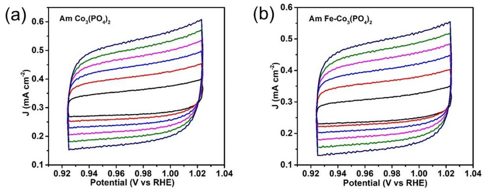
**Fig. S9** Cyclic voltammograms of (a) Am Co<sub>3</sub>(PO<sub>4</sub>)<sub>2</sub> and (b) Am Fe-Co<sub>3</sub>(PO<sub>4</sub>)<sub>2</sub> with a potential window from 0.924 to 1.024 V at different scan rates in 1.0 M KOH.
