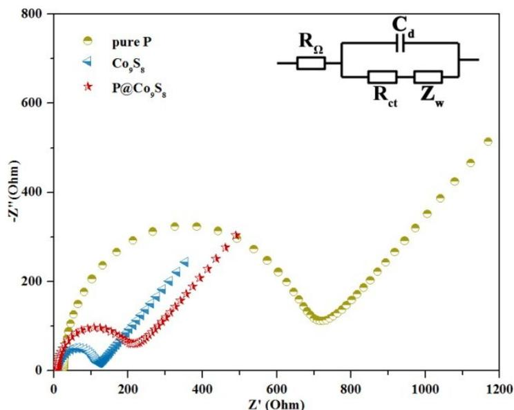
**Figure S5** Electrochemical impedance spectroscopy of P,  $\text{Co}_9\text{S}_8$  and  $\text{P@Co}_9\text{S}_8$ .
