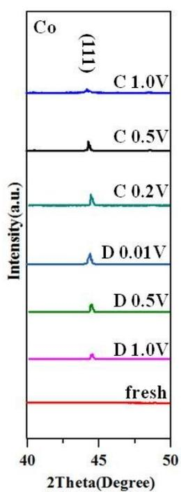
**Figure S4** The *ex-situ* XRD of the discharge-charge profile of P@Co<sub>9</sub>S<sub>8</sub> at different potentials for the 1<sup>st</sup> cycle at current density of 0.5 A g<sup>-1</sup>.
