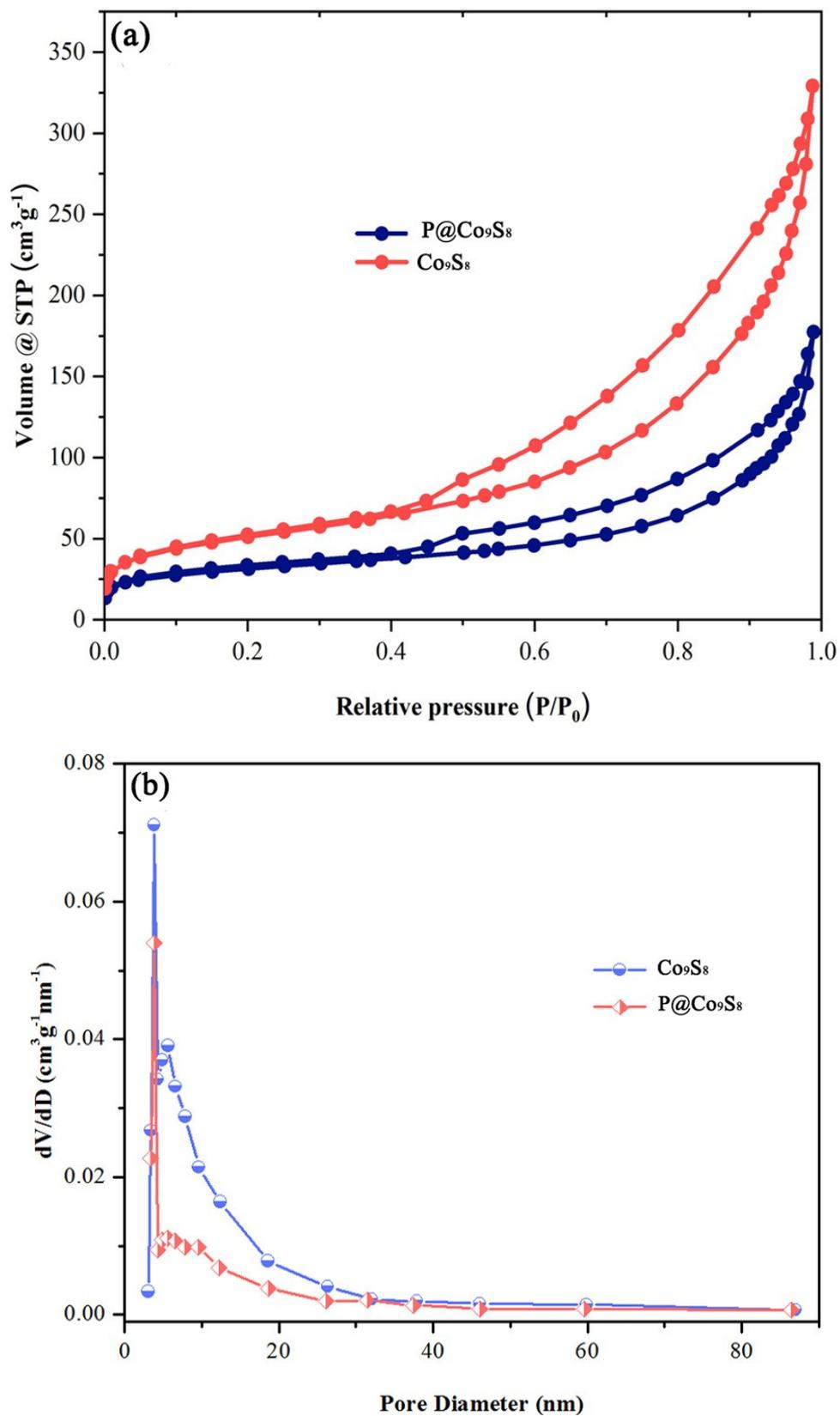
**Figure S2** (a) Nitrogen adsorption-desorption isotherms, (b) Pore size distribution of  $\text{P@Co}_9\text{S}_8$  and  $\text{Co}_9\text{S}_8$ .
