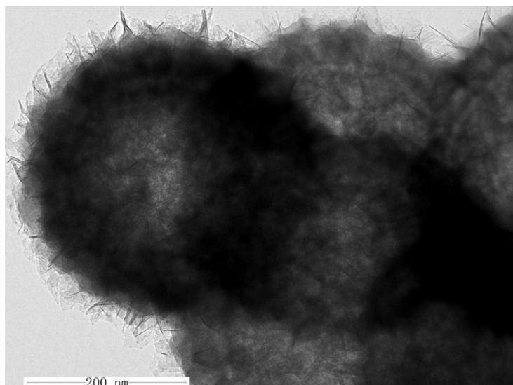
**Figure S3** Detailed TEM image of P@Co<sub>9</sub>S<sub>8</sub> electrode after 1000 cycles.
