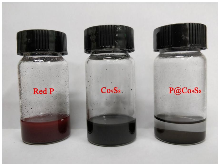
**Figure S1.** The solubility of red P,  $\text{Co}_9\text{S}_8$  and  $\text{P@Co}_9\text{S}_8$  in the liquid electrolyte.
