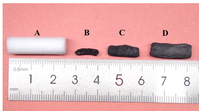
Fig. S1. Photograph of samples (A) CF, (B) carbonised GO ( 1 \text{ mg mL}^{-1} )@CF, (C) carbonised GO ( 5 \text{ mg mL}^{-1} )@CF, and (D) carbonised GO ( 10 \text{ mg mL}^{-1} )@CF.
