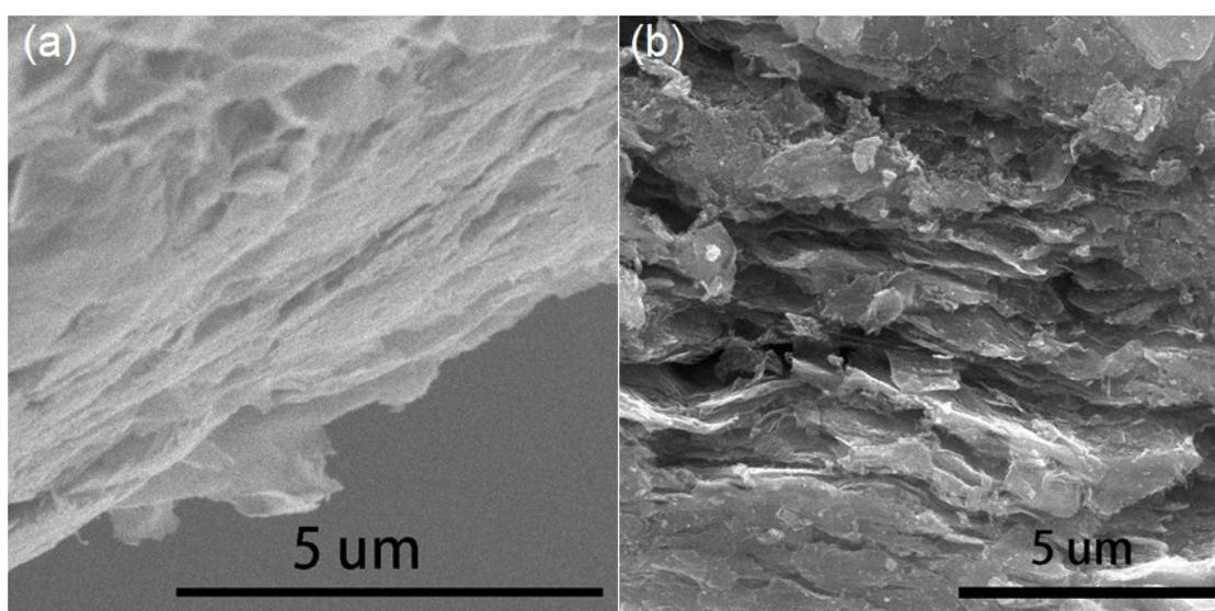
**Figure S3** SEM images of purity  $Ti_3C_2T_x$  (a) and (b)  $Ti_3C_2T_x$  treated by RhB.
