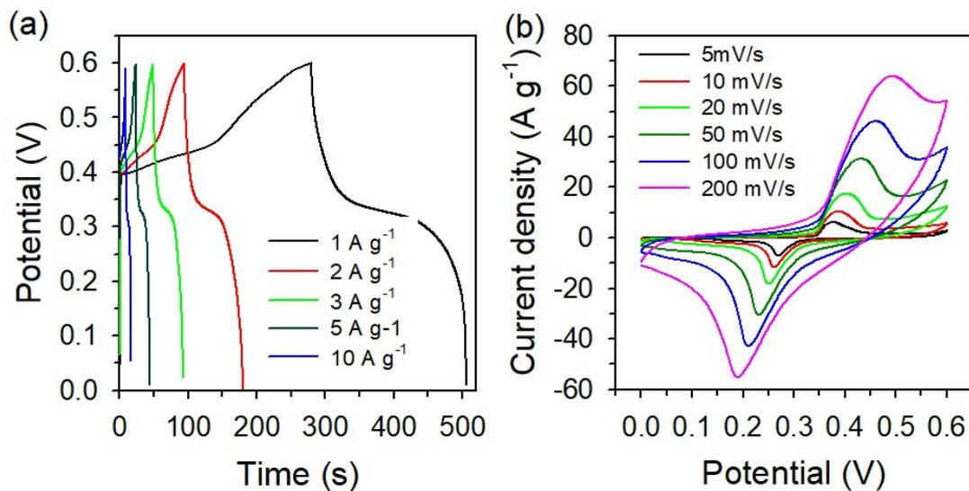
**Figure S4** Three electrode (a) GCD curves of the TRhB-600 electrode at current densities of 1, 2, 3, 5 and 10 A g<sup>-1</sup>, respectively. (b) CV curves of the TRhB-600 electrode at scan rates of 5, 10, 20, 50, 100 and 200 mV s<sup>-1</sup>.
