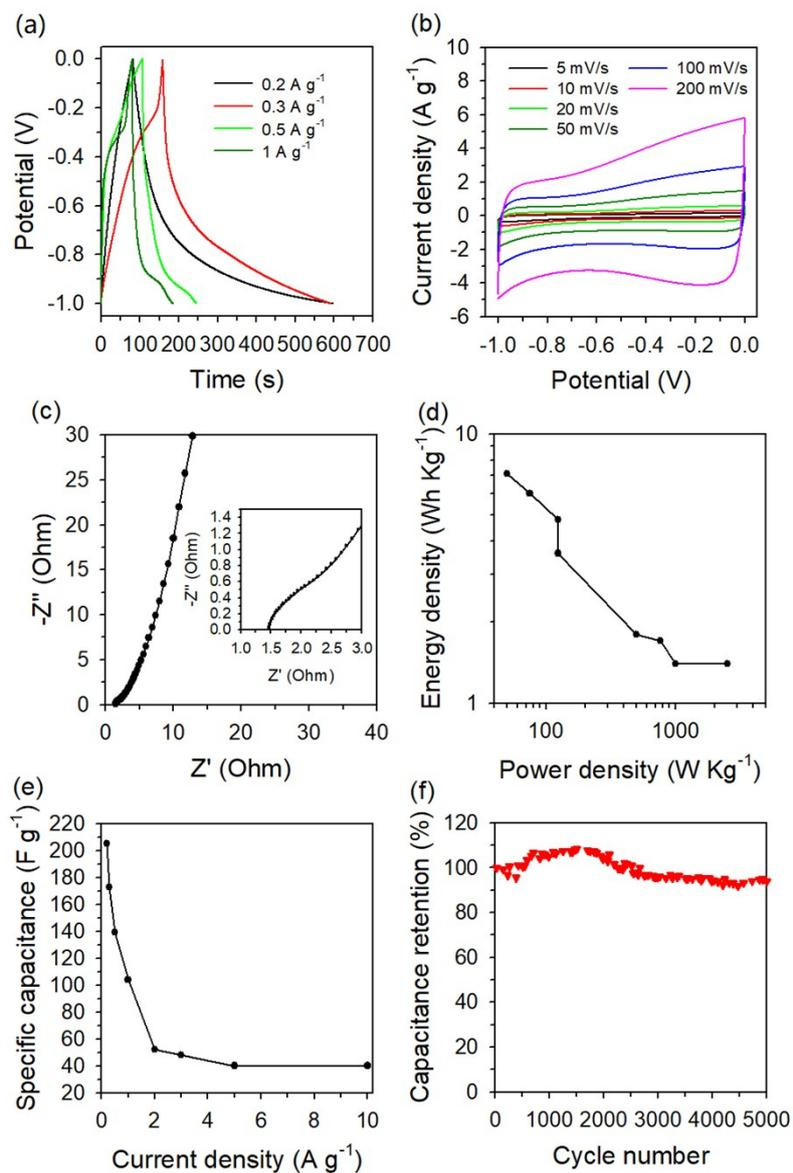
**Figure S5** 6 M KOH as electrolyte in two-electrode system (a) GCD curves of TRhB-600 electrode at various current density; (b) CV curves of TRhB-600 electrode at various scanning rates; (c) EIS for TRhB-600 electrode; (d) Ragone plot of TRhB-600 electrode; (e) Rate performance of TRhB-600 electrode as a function of scan rate; and (f) cycling stability of TRhB-600 at 3 A g<sup>-1</sup> over 8000 cycles.
