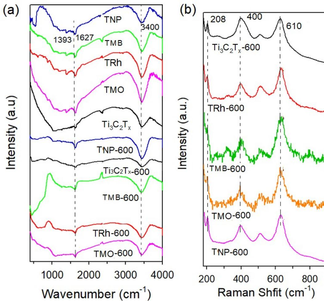
**Figure S2** (a) IR transmission spectra of all samples at room temperature in KBr wafer. (b) Raman spectra of TC-600, TMO-600, TMB-600, TR-600, and  $Ti_3C_2T_x$ -600.
