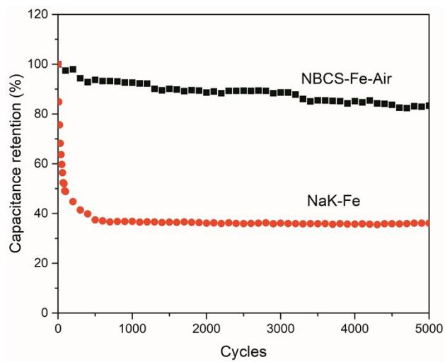
**Fig. S2** Cycling stability of NBCS-Fe-Air and NaK-Fe at  $5 \text{ A g}^{-1}$  in the three-electrode system.
