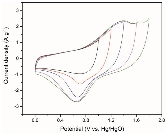
**Fig. S5** CV curves of the NBCS-Fe-Air//FMO asymmetric supercapacitor collected in various potential windows at  $30 \text{ mV s}^{-1}$ .
