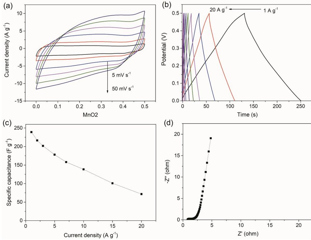
**Fig. S4** Electrochemical performance of FMO in a three-electrode system. (a) CV curves at different scan rates, (b) GCD curves at different current densities, (c) specific capacitance of the samples as a function of current density and (d) Nyquist plots.
