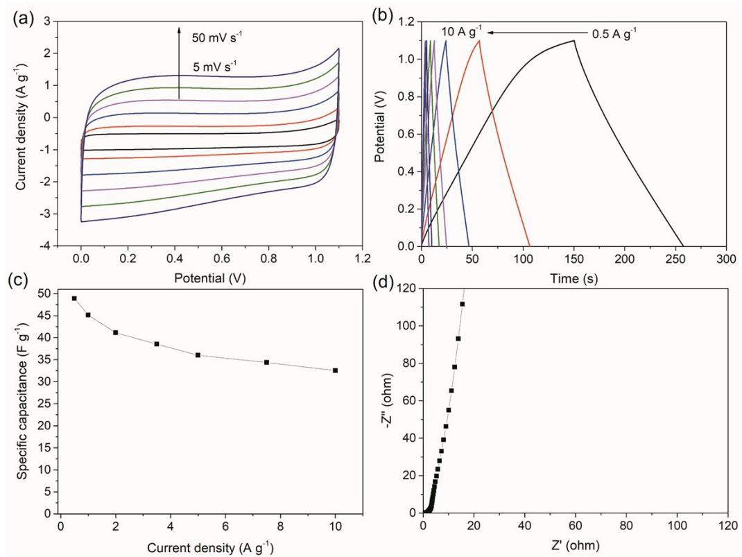
**Fig. S3** Electrochemical performance of NBCS-Fe-Air in a symmetrical two-electrode system. (a) CV curves at different scan rates, (b) GCD curves at different current densities, (c) specific capacitance of the samples as a function of current density and (d) Nyquist plots of NBCS-Fe-Air//NBCS-Fe-Air symmetrical supercapacitor.
