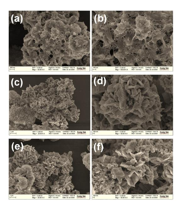
**Figure S1.**  $\beta$ -NiS products prepared at fixed reaction time (12 h) and various temperature conditions such as (a) & (b) 150 °C, (c) & (d) 160 °C and (e) & (f) 180 °C.
