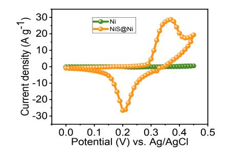
Figure S2. CV comparison of NiS@Ni with Ni foam at the scan rate of 10 mV s<sup>-1</sup>.
