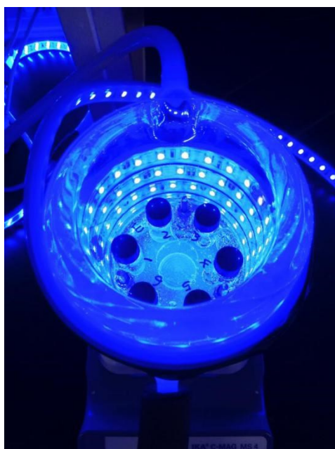
Figure S3. Image of homemade photoenzymatic decarboxylation reaction setup used in the experiment [3] .
