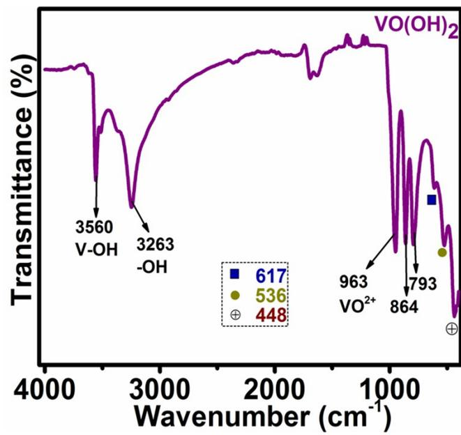
Fig. S1 FTIR spectra of  $\text{VO}(\text{OH})_2$ .
