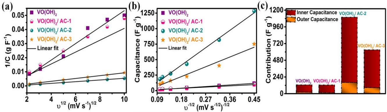
Fig. S6 (a, b, c) Trasatti plot for  $\text{VO}(\text{OH})_2$ ,  $\text{VO}(\text{OH})_2/\text{AC}-1$ ,  $\text{VO}(\text{OH})_2/\text{AC}-2$ ,  $\text{VO}(\text{OH})_2/\text{AC}-3$ .
