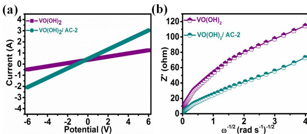
Fig. S4 (a) I-V measurement of  $\text{VO}(\text{OH})_2$ ,  $\text{VO}(\text{OH})_2/\text{AC}-2$  (b) Randles plot of  $\text{VO}(\text{OH})_2$ ,  $\text{VO}(\text{OH})_2/\text{AC}-2$ .
