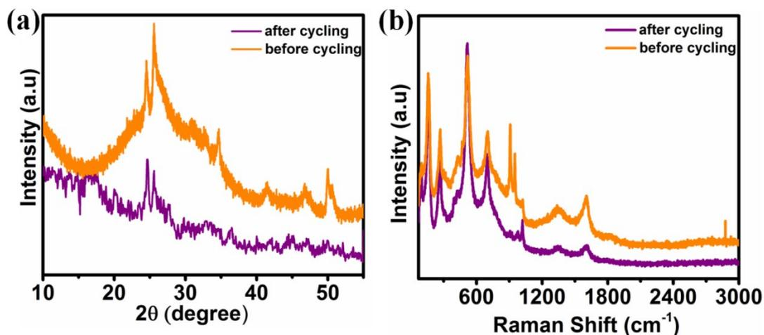
Fig. S7 (a) XRD, (b) Raman spectra of VO(OH)<sub>2</sub>/AC-2 before and after cycling.
