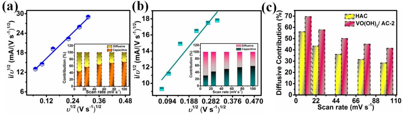
Fig. S5 Plot of  $1/v^{1/2}$  versus  $v^{1/2}$  for: (a) HAC (b)  $\text{VO}(\text{OH})_2/\text{AC}-2$  (c) Contribution of diffusive current at  $-0.2$  V.
