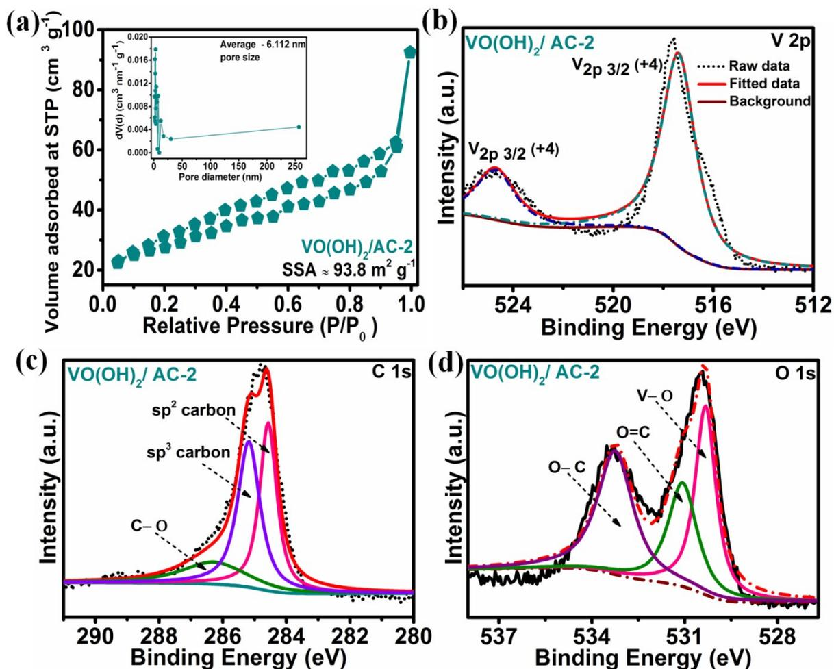
Fig. S3 (a) Nitrogen sorption isotherms [inset: Pore size distribution] XPS spectra of (b) V 2p (c) C 1s (d) O 1s of VO(OH)<sub>2</sub>/AC-2.
