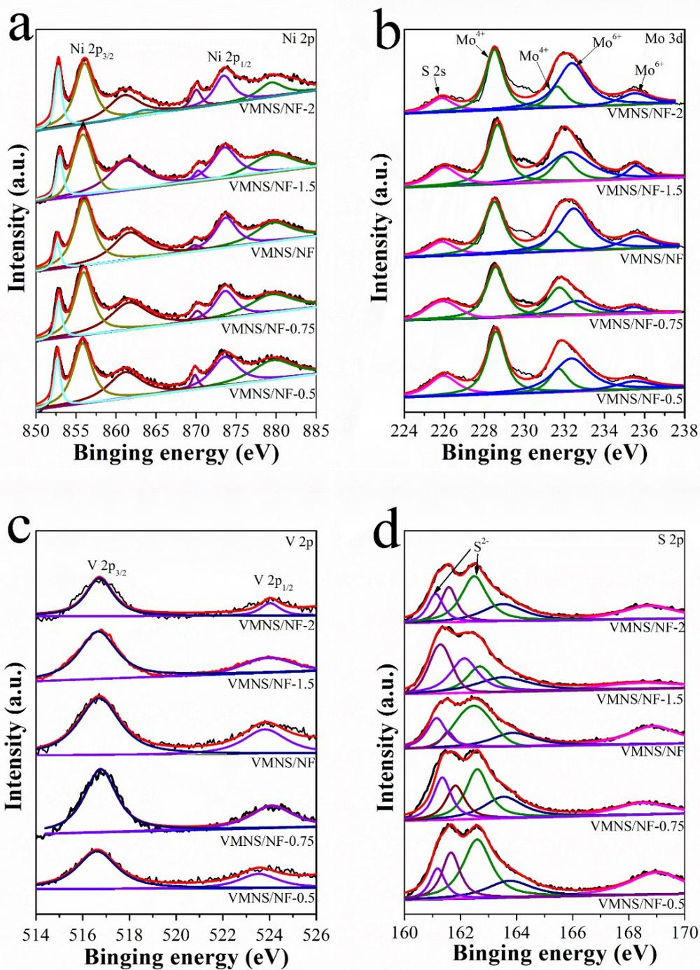
**Fig. S5** XPS spectra of the VMNS/NF- $\beta$  ( $\beta = 0.5, 0.75, 1, 1.5, 2$ ): (a) Ni 2p, (b) Mo 3d, (c) V 2p, and (d) S 2p spectrum.
