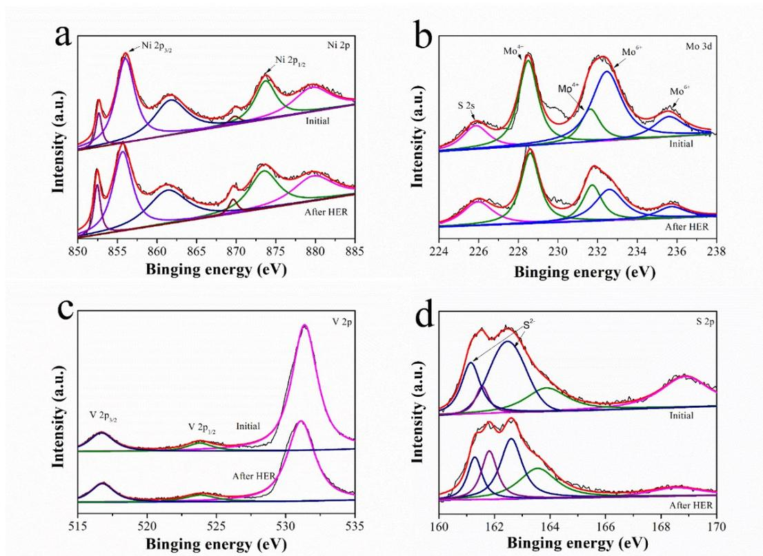
**Fig. S9** XPS spectra of the VMNS/NF after HER reaction: (a) Ni 2p, (b) Mo 3d, (c) V 2p, and (d) S 2p.
