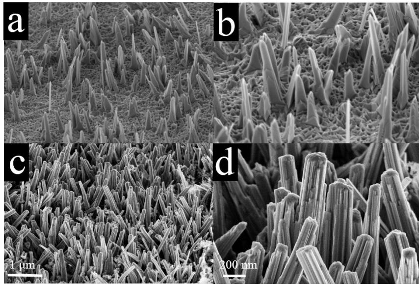
**Fig. S3** (a and b) SEM images of the NS/NF; (c and d) SEM images of the VNS/NF.
