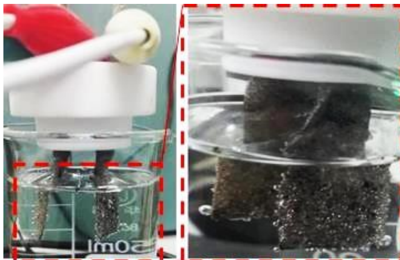
Figure S16. Optical photographs of electrocatalytic water splitting process, showing (a) the three electrode glass cell and bubbles on the surface of working electrode.
