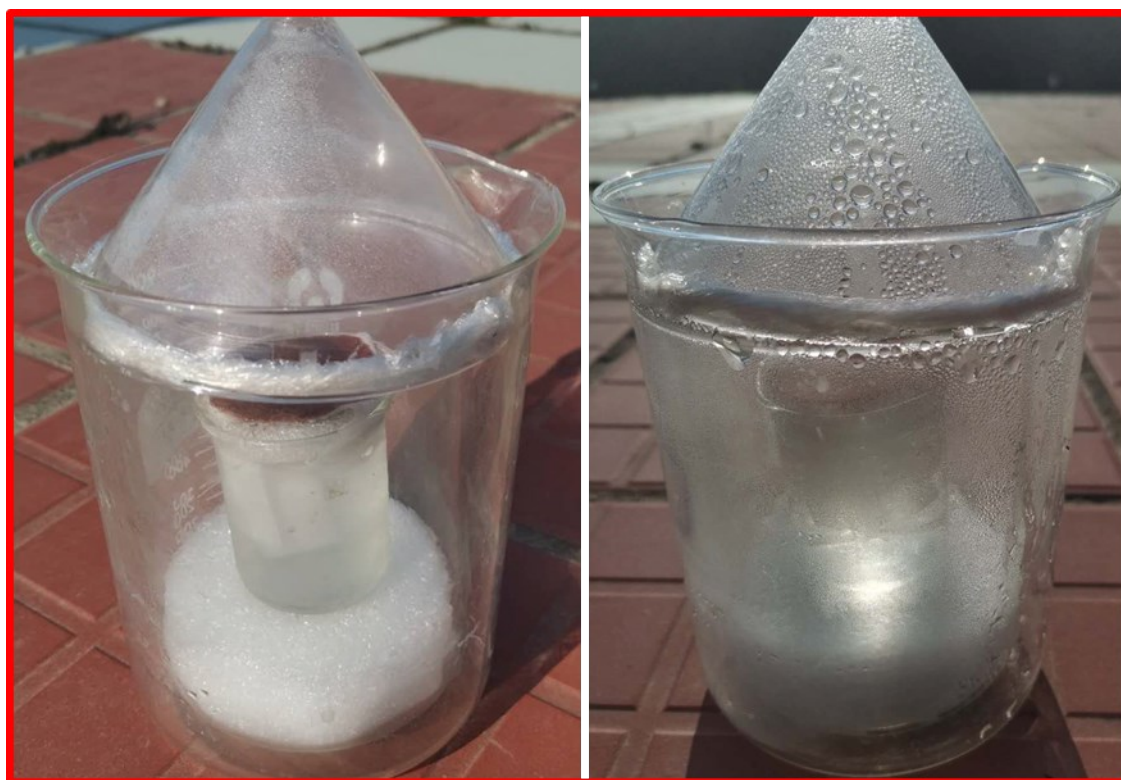
Fig. S8. The fresh water collection device based on Mn-MCM under natural light.
