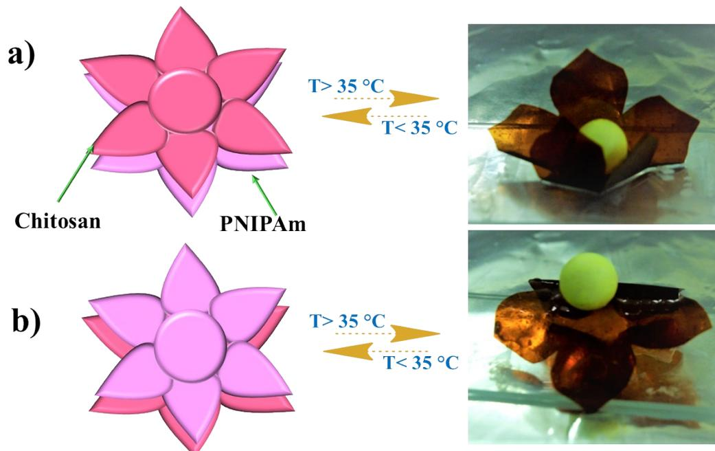
**Figure S4:** Temperature-induced actuation performance of chitosan/pNipam bilayer. a) optical images of six petal-shaped chitosan flower when pNipam coating at the bottom side. The image at the right-hand side shows the folded structure showing the gripping; b) pNipam coating on the top side of the petals represents the soft cargo application.
