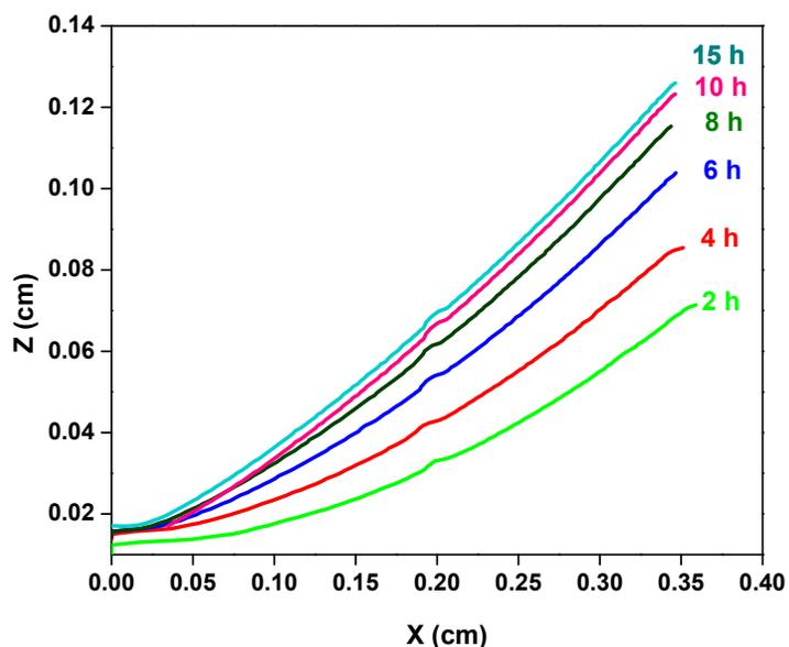
**Figure S3:** Plot showing reusability of the bilayer by retaining the triggering solvent by pNipam microgels. The graph displays the configuration in X-Z plane of the bilayer, here the folding is achieved by placing the bilayer at 1.5 °C for different time intervals.
