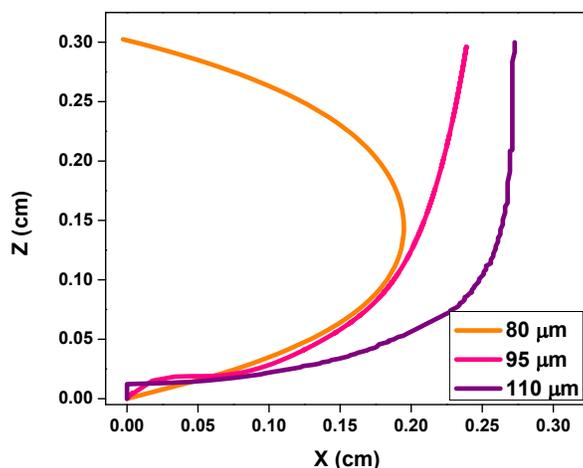
**Figure S1:** Plot of the X and Z displacements for different thickness of chitosan layer. As observed the folding reduces with the increase of film thickness.
