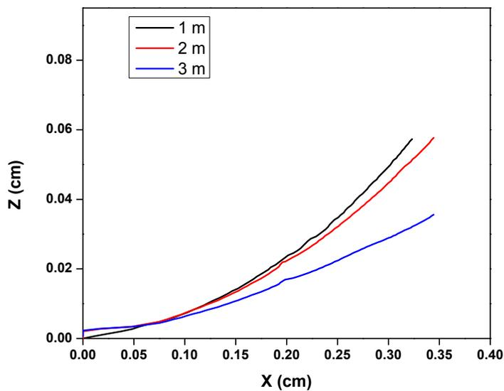
**Figure S2:** Plot represents X and Z displacements using different molar resorcinol loaded pNipam particles.
