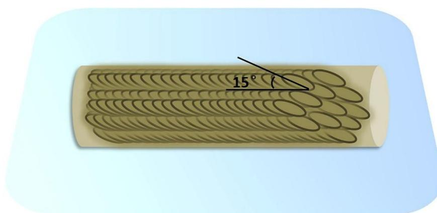
**Figure S14.** Scheme of the orientation of the discotic molecular in the microfiber.
