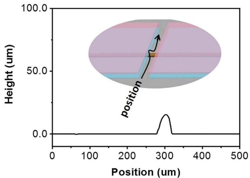
**Figure S15.** The typical step profiler analysis for determination of the cross-sectional area of the microfiber.
