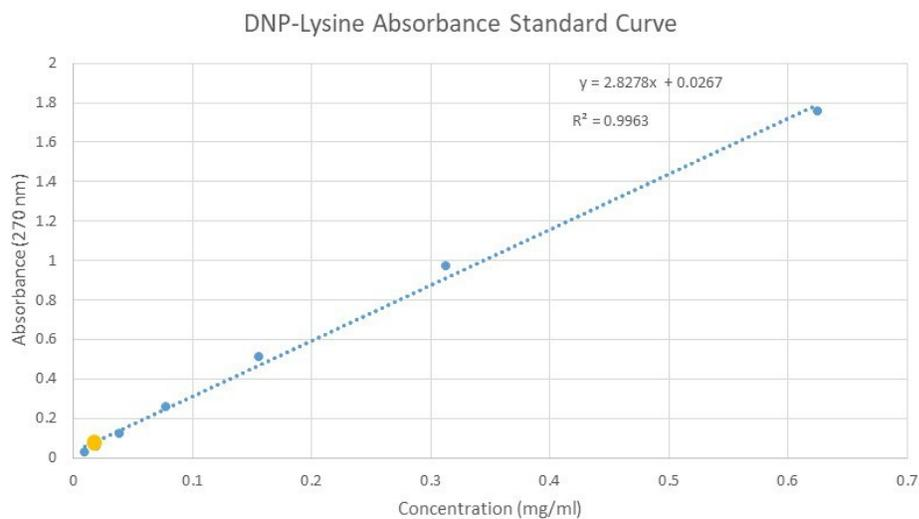
**Fig. S2** Standard curve of absorbance (wavelength = 270 nm) of DNP-lysine. Absorbance of 0.5 mg/mL of polymer-peptide conjugate shown in orange, corresponding to 95% conjugation efficiency.
