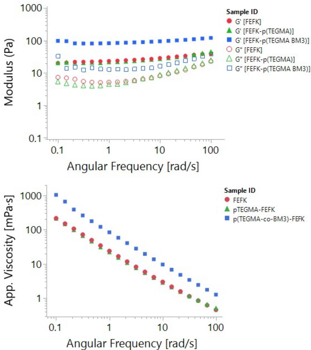
**Fig. S3** Rheology studies for hydrogels formed without sodium hydroxide (pH ~4). Frequency sweep (left) and viscosity profile (right) of 20 mg/mL solutions of FEFK-p(TEGMA BM3), FEFK-p(TEGMA), and pure FEFK gels at 2.5% wt. For each gel, the data represents two replicates averaged together.
