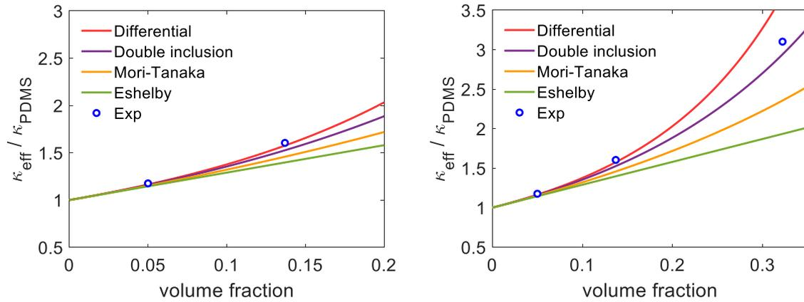
Fig. S3. Different homogenization models for effective thermal conductivities of LMCs when the thermal conductivity of the PDMS is increased by 10% from the experimental data.
