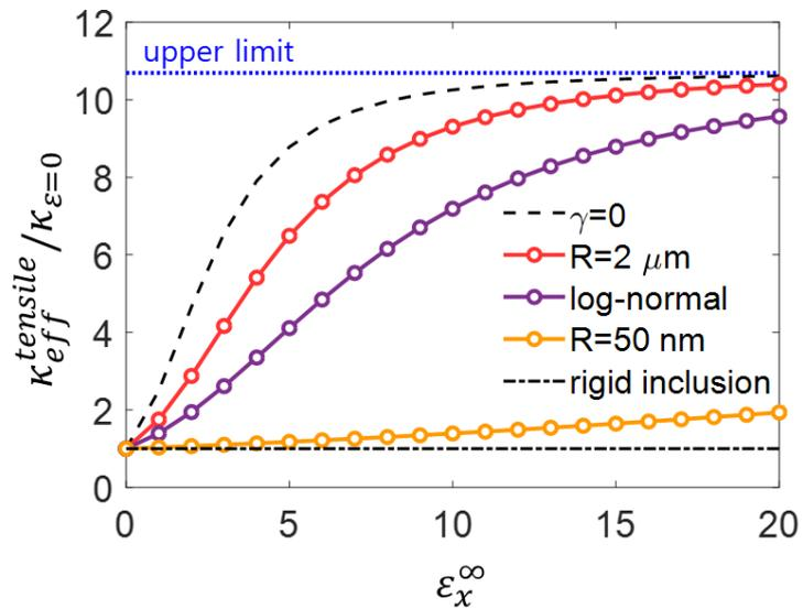
Fig. S4. Effective thermal conductivities in the tensile direction under the far field strain at 20% of volume fraction. Thermal conductivities are normalized by thermal conductivity at zero strain.
