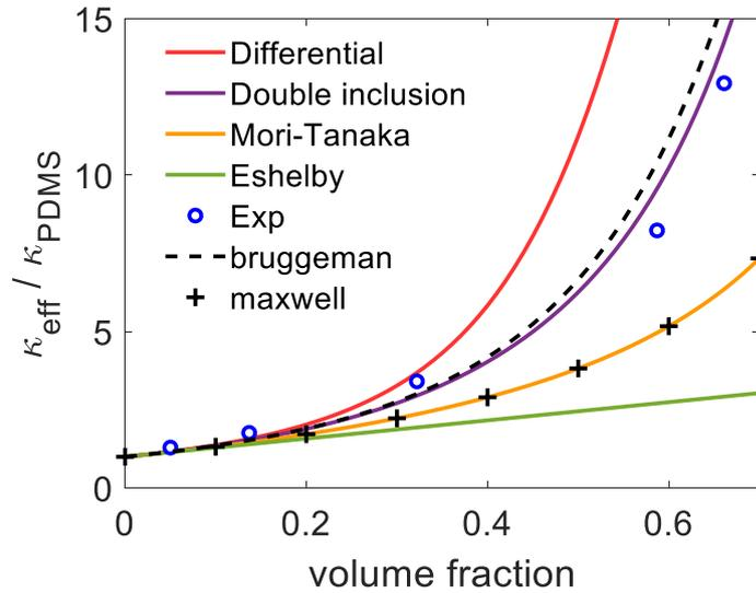
Fig. S1. Different homogenization models for effective thermal conductivities of LMCs. Predictions from Maxwell-Garnett's model and Bruggeman's theory are added. The thermal conductivities are normalized by the thermal conductivity of PDMS.
