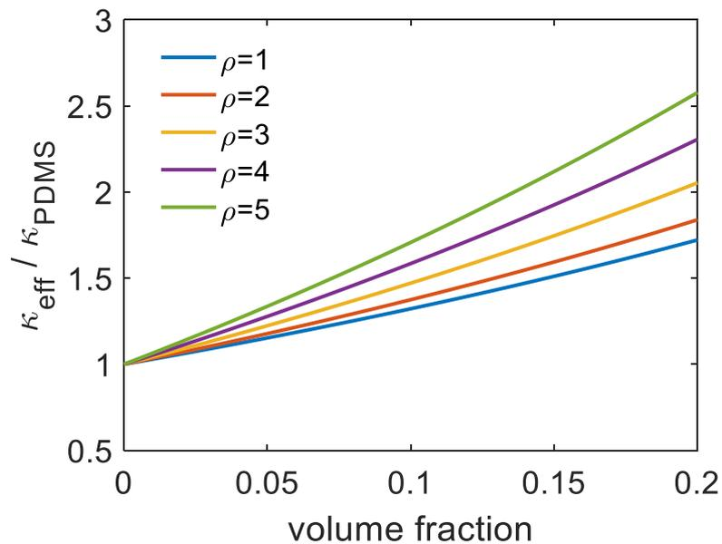
Fig. S2. Normalized effective thermal conductivities of LMCs when aspect ratios are 1, 2, 3, 4 and 5, respectively. Ellipsoidal LM inclusions are randomly oriented.
