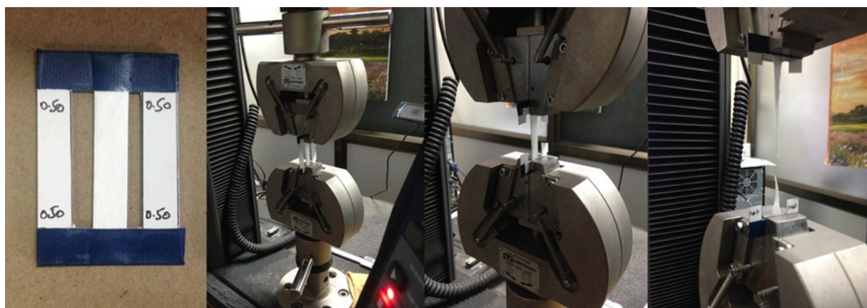
Figure S1 Tensile testing of electrospun fabrics.
