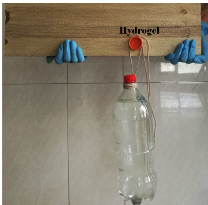
Figure S5. Adhesive ability of the SNDCL hydrogel lifting a 2 kg bottle of water.
