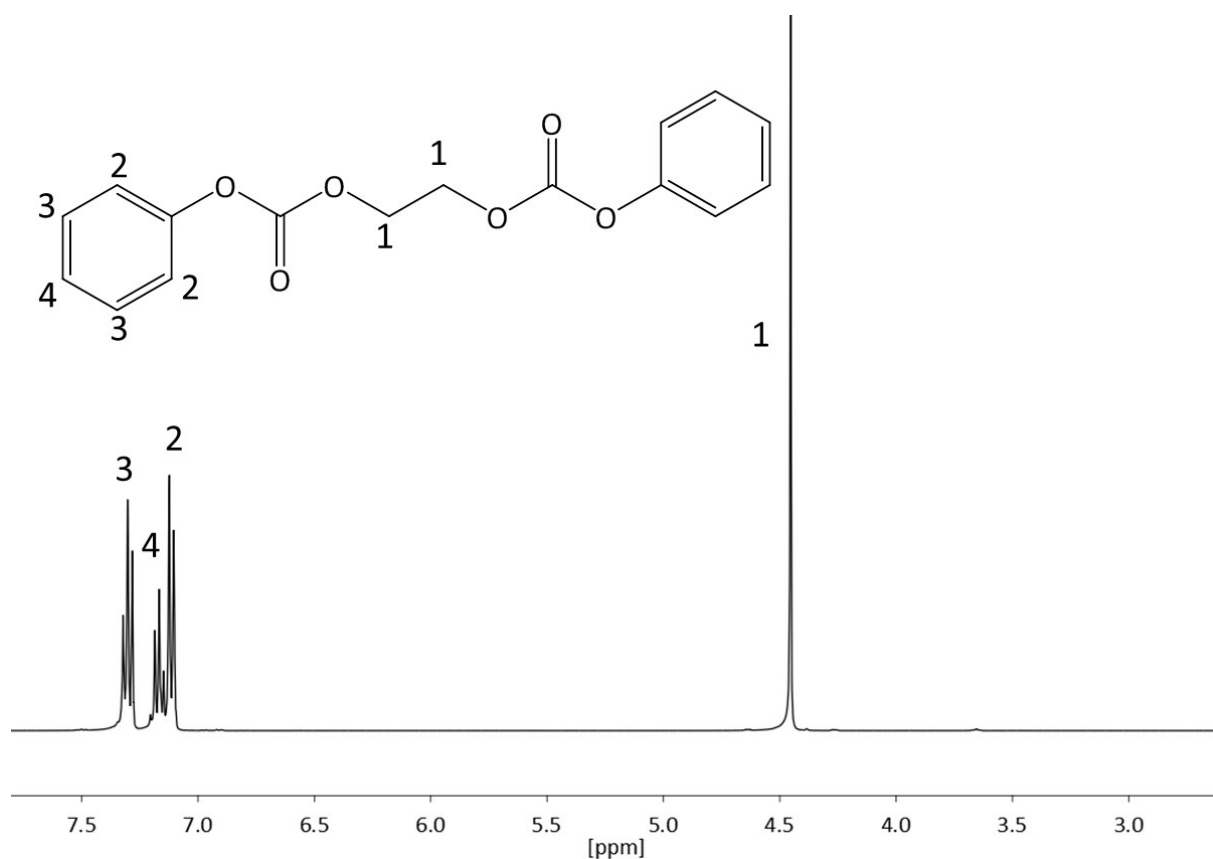
Figure S3. Proton NMR spectra of phenylcarbonate telechelic ethylene glycol in CDCl 3 .
