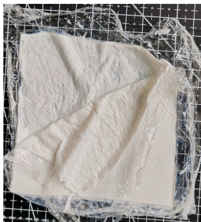
Figure S3 The photo of the half-separated PP films (the film between solution and glass mode to prevent the adhesion of the polymerized product on the glass mode) and the product after the polymerization of MAA in Gel/MAA solution with 8 wt % MAA at 30 °C.
