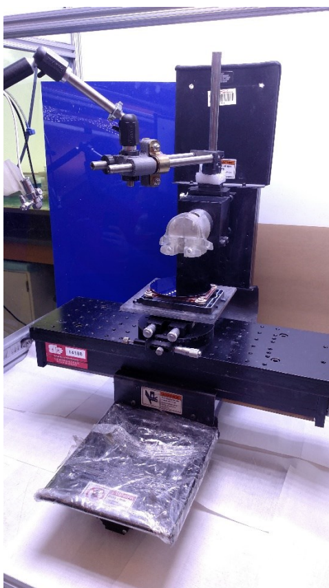
Figure S4. The 3D printing stage. Syringe barrels full of ink are loaded into the white plastic clip to be printed. Extrusion is driven by the Nordson Ultimius V pressure actuator (out of frame).
