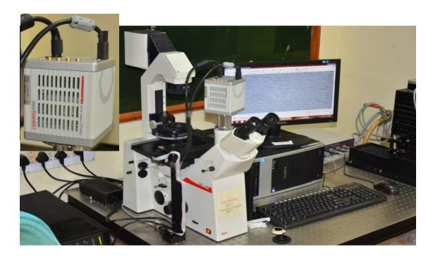
For microscopy, the source of the magnetic field was a permanent magnet sitting on two arms of a motorized stage, which was brought closer to the sample using a stepper motor. For microscopy, the source of the magnetic field was a permanent magnet sitting on two arms of a motorized stage, which was brought closer to the sample using a stepper motor.
