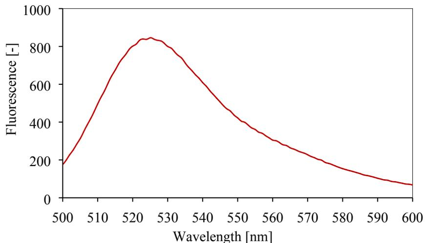
Fig. SI 3: Fluorescence emission spectrum of CA IX-F, excitation 488 nm.
