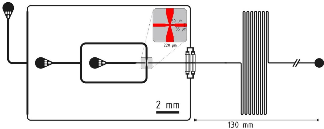
Fig. SI 4: The layout of the 1<sup>st</sup> generation chip with a combined gelation and extraction part
