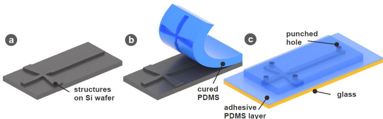
Fig. SI 1: Fabrication process of the microfluidic chip: a) silicon master with designed structures, b) cured PDMS replica, c) assembled microfluidic chip
