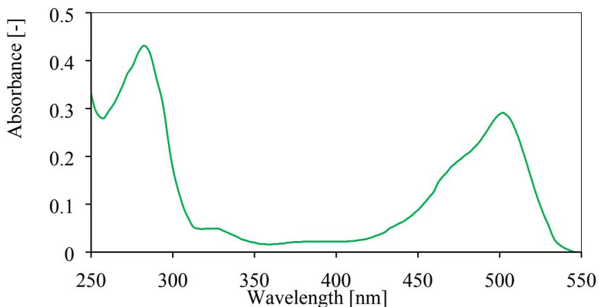
Fig. SI 2: Absorption spectrum of CA IX-F with concentration 0.4 mg/mL.
