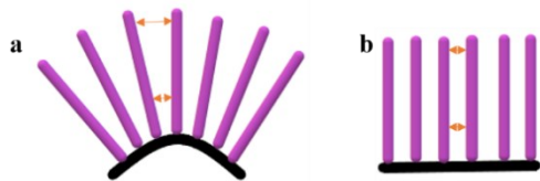
Figure S4 - a schematic representation of the effect of the membrane curvature on the alignment of the perpendicular fibers
