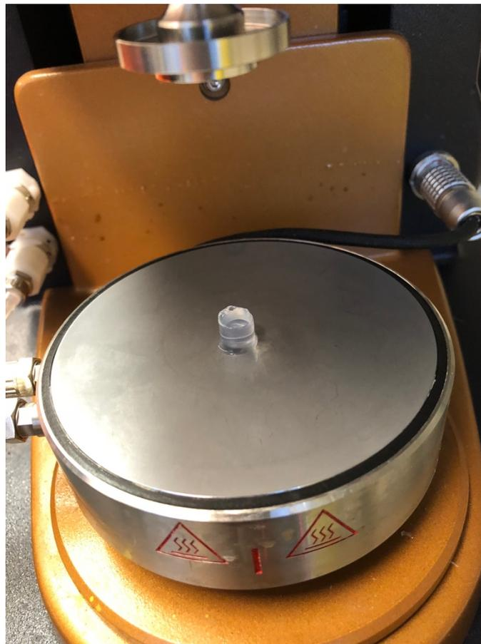
**Figure S7.** An image of an Fmoc-F5-Phe 5 mM gel which was set beforehand and transferred to the plate. This image is taken before the foot is lowered and the gap set.
