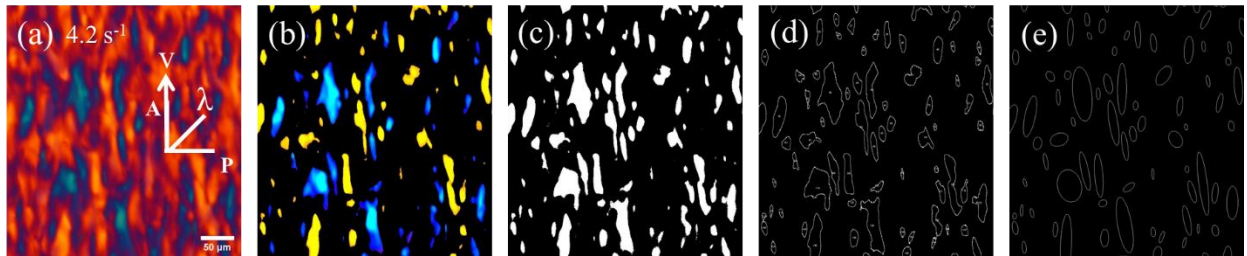
Fig. S2. Identification of domain structure and determination of a_x and a_y in Region II. (a) POM texture with FWP and crossed polarizers; (b) blue and yellow domains selected using Fiji2/ImageJ color threshold 2 , (c) binary image of part (b), (d) outlines of the domains, and ellipses fitting the domains in panel (d), obtained by using Analyze Particles in Fiji2/imageJ 2 . Projections of the two axes of the ellipses onto the directions of flow and vorticity define a_x and a_y , respectively.
