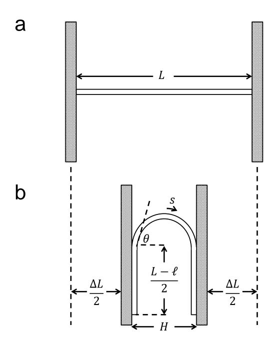
FIG. 1. Geometry of a tape loop. a. before compression of the walls, the film of length L lies flat. b. shows the film after some compression of the walls.
