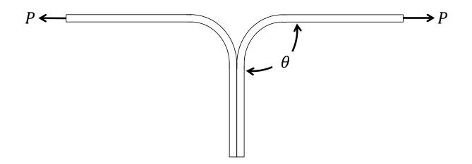
FIG. 2. Geometry of a T-Peel test.
