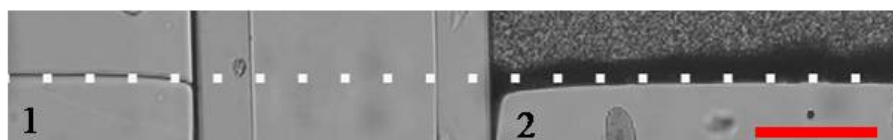
Figure 1: Interface positions of freezing deionized water (left sample 1) and freezing suspensions (right sample 2) under the identical thermal gradient. The lower part is cooling zone and the higher part is heating zone. The white dotted lines are their interface positions. The red scale bar is 150\ \mu\text{m} .
