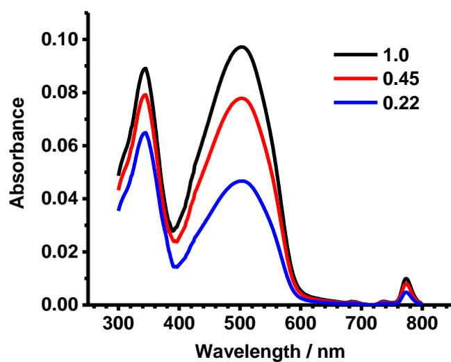
**Figure S12.** UV-visible spectra for labelled DXMG-GMA gel obtained at various compressive compression deformation ratios.
