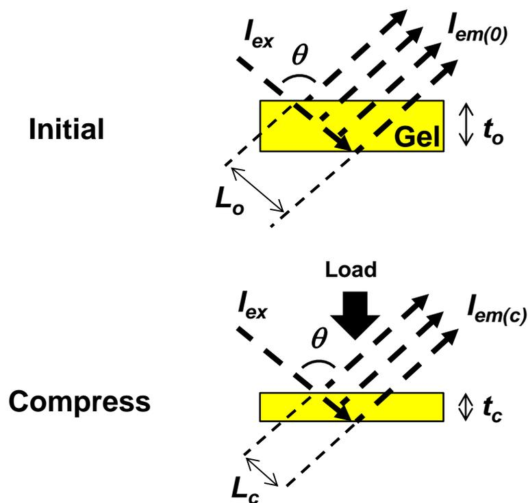
**Figure S8.** Geometry for a PL experiment involving a gel before and during compression.
