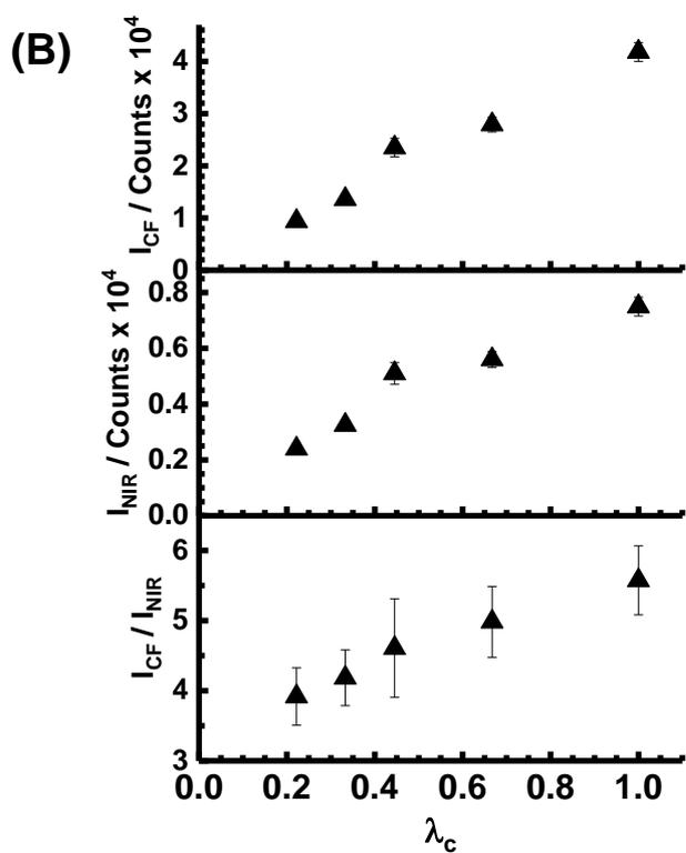
**Figure S7.** (A) As-measured PL spectra for labelled PEI-MG during compression. The compression deformation ratios ( $\lambda_c$ ) are shown in the legend. (B) Variation of  $I_{CF}$ ,  $I_{NIR}$  and  $I_{CF}/I_{NIR}$  with  $\lambda_c$ . The error bars for some of the points in (B) are smaller than the symbols.
