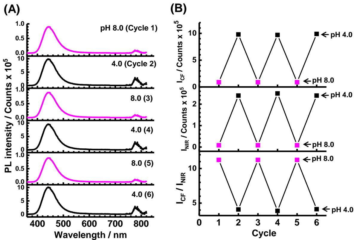
**Figure S6.** (A) PL spectra and (B) PL intensity of the CF and NIR peaks at pH 4.0 and 8.0 for labelled DXMG-GMA gel measured during pH switching.
