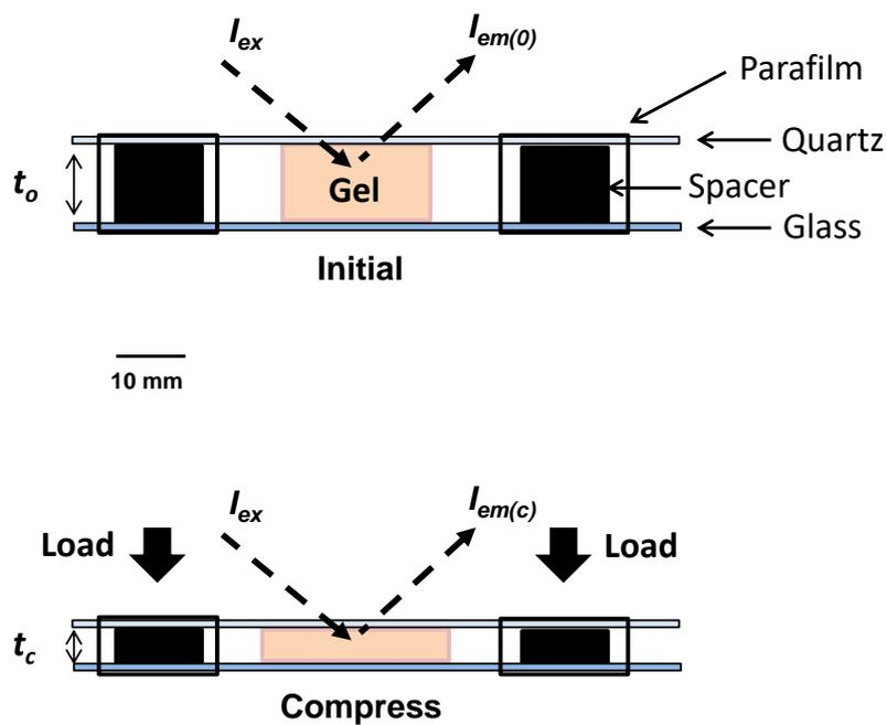
**Figure S1.** Schematic diagram showing how the gels were compressed whilst measuring the PL emission spectra.  $I_{ex}$  and  $I_{em}$  are the intensities of the excitation and emission beams.
