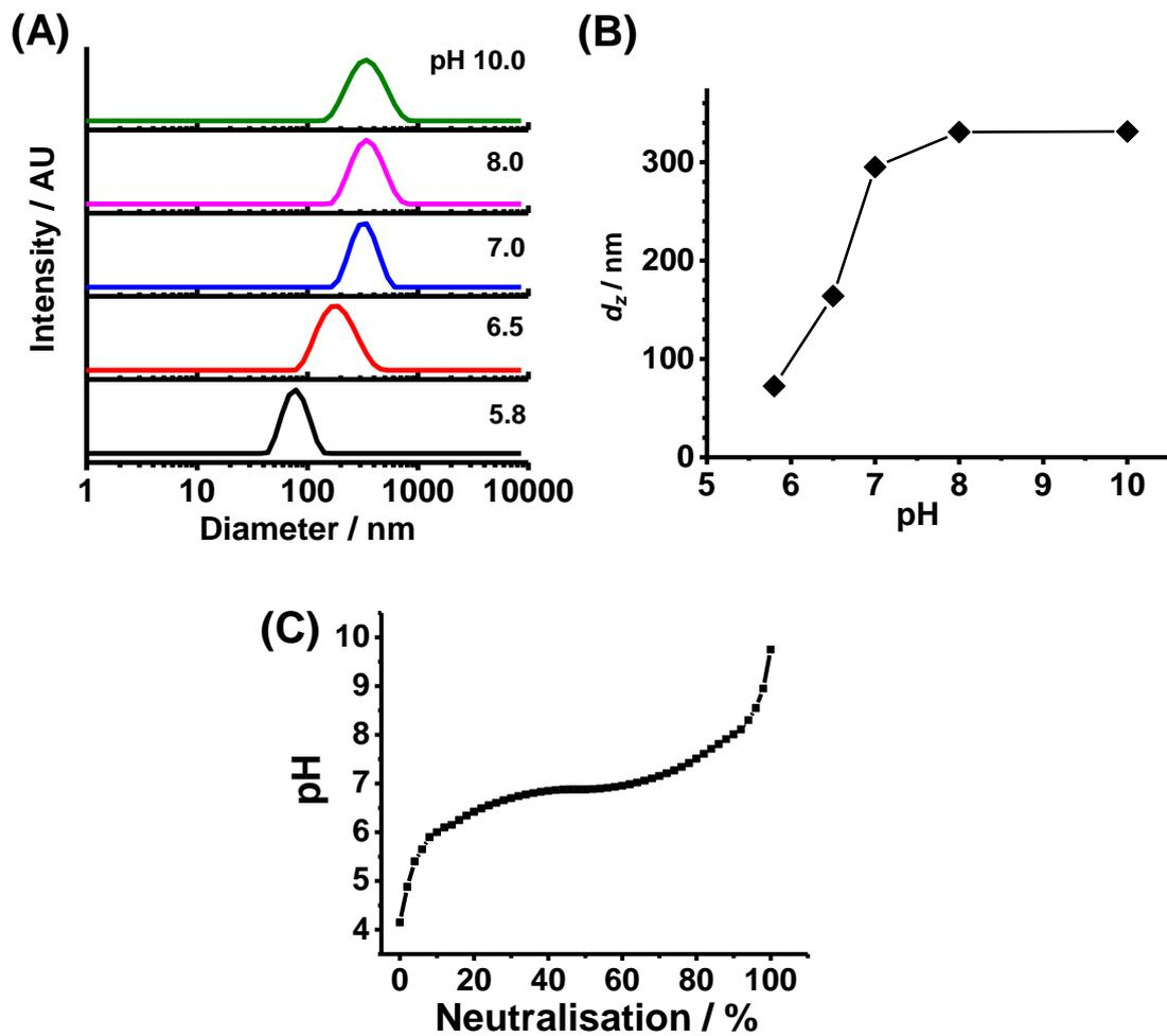
**Figure S2** DLS size distributions (A) and z-average diameter as a function of pH (B) for the CF particles. (C) Titration data for the CF dispersion.
