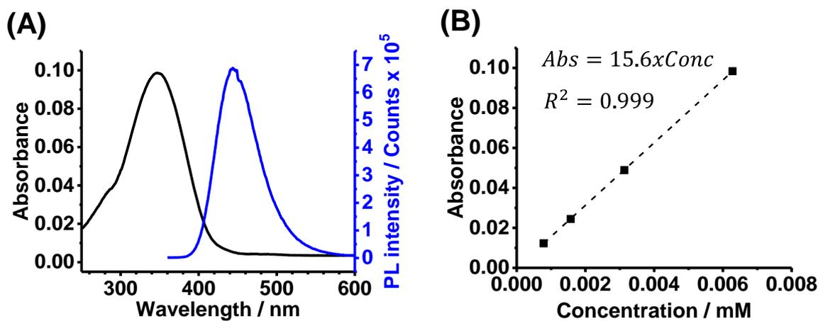
**Figure S3** (A) UV-visible and PL spectra for CF350. (B) Concentration dependence of the absorbance measured at the absorption maximum in (A). The molar extinction coefficient was calculated as  $1.56 \times 10^4 \text{ mol}^{-1} \text{ dm}^3 \text{ cm}^{-1}$ . The latter value is within 85% of the value provided by the supplier<sup>1</sup>.
