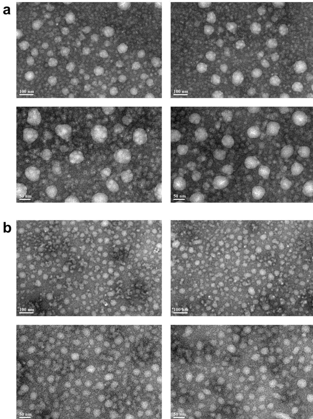
Figure S9. Additional TEM images of NS-1 at different temperatures after negative staining with phosphotungstic acid. (a) 20 °C, (b) 60 °C.
