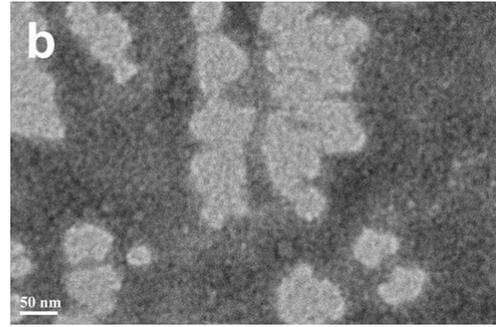
Figure S6. TEM images of non-complementary ELP-ON conjugates after negative staining with phosphotungstic acid. (a) ELP-ON5, (b) ELP(ON2-ON5) mixture.
