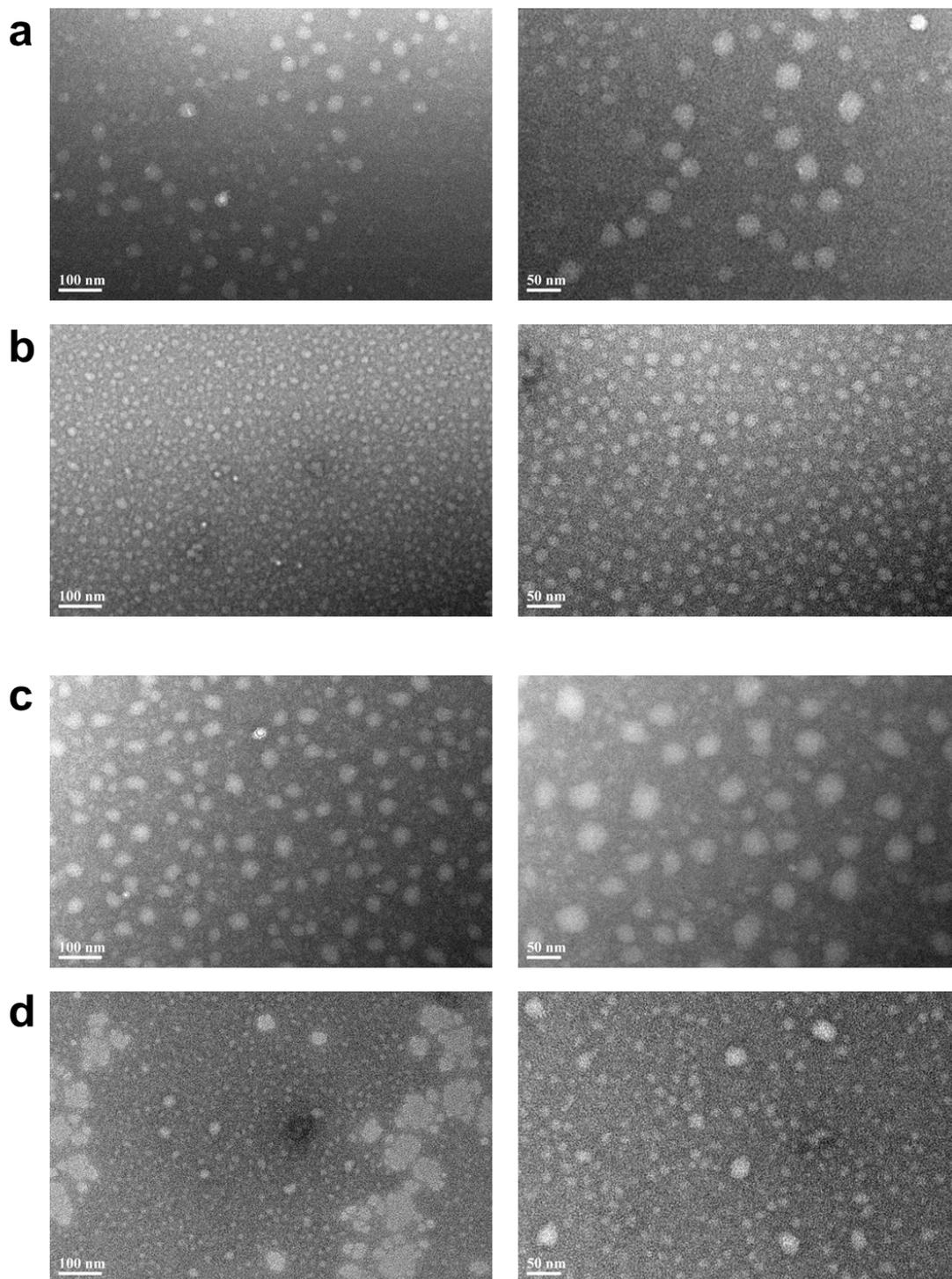
Figure S11. TEM images of NSs in 2 mM  $Mg^{2+}$  at different temperatures after negative staining with phosphotungstic acid. (a) NS-1 at 20 °C, (b) NS-1 at 60 °C, (c) NS-2 at 20 °C, (d) NS-2 at 60 °C.
