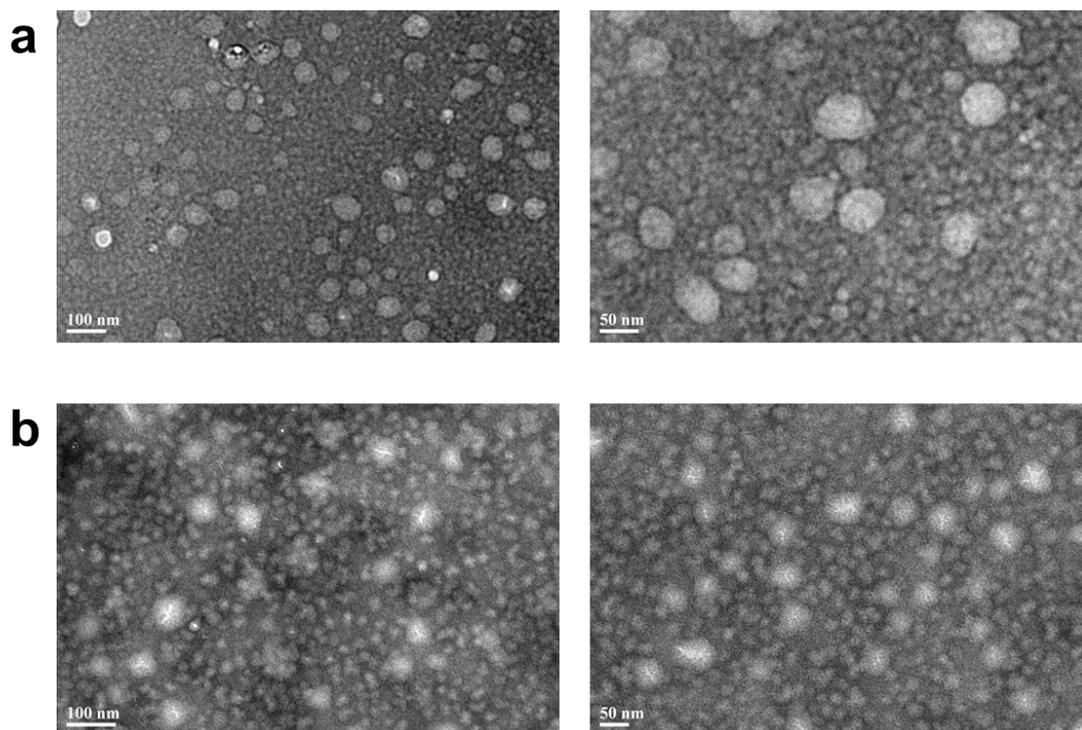
Figure S4. TEM images of NSs at room temperature after negative staining with phosphotungstic acid. (a) NS-1, (b) NS-2.
