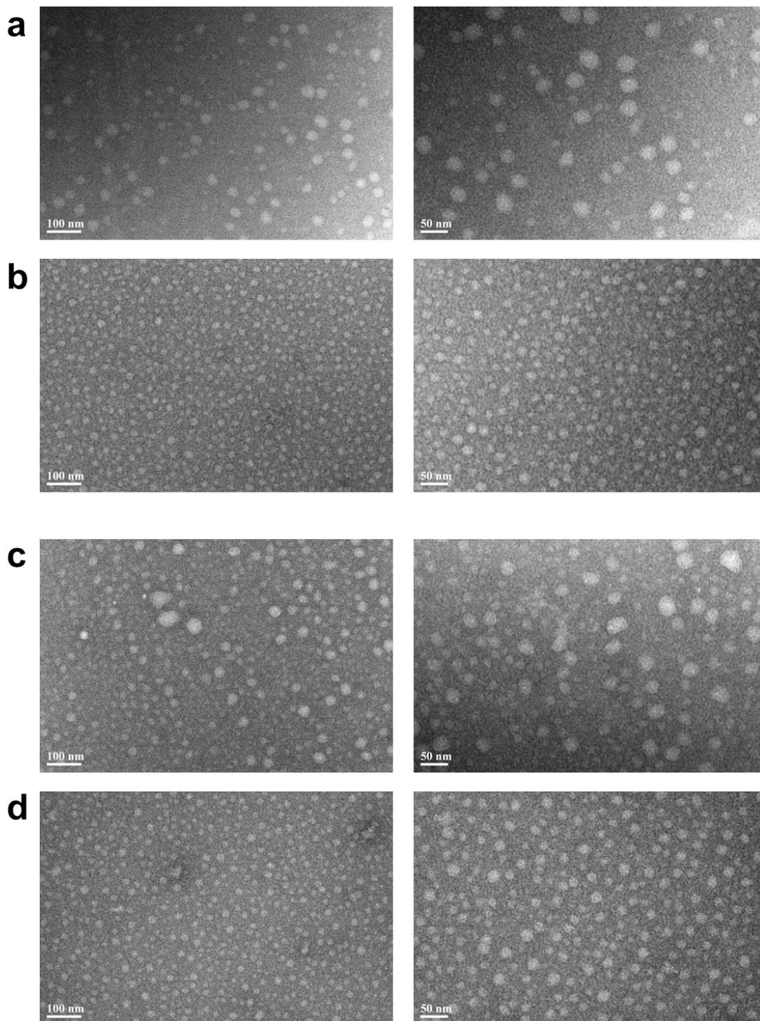
Figure S12. TEM images of NSs in 25 mM  $Mg^{2+}$  at different temperatures after negative staining with phosphotungstic acid. (a) NS-1 at 20 °C, (b) NS-1 at 60 °C, (c) NS-2 at 20 °C, (d) NS-2 at 60 °C.
