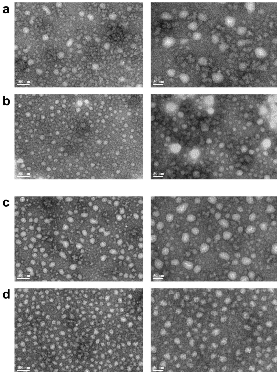
Figure S13. TEM images of NSs in the absence of  $\text{Mg}^{2+}$  at different temperatures after negative staining with phosphotungstic acid. (a) NS-1 at 20 °C, (b) NS-1 at 60 °C, (c) NS-2 at 20 °C, (d) NS-2 at 60 °C.
