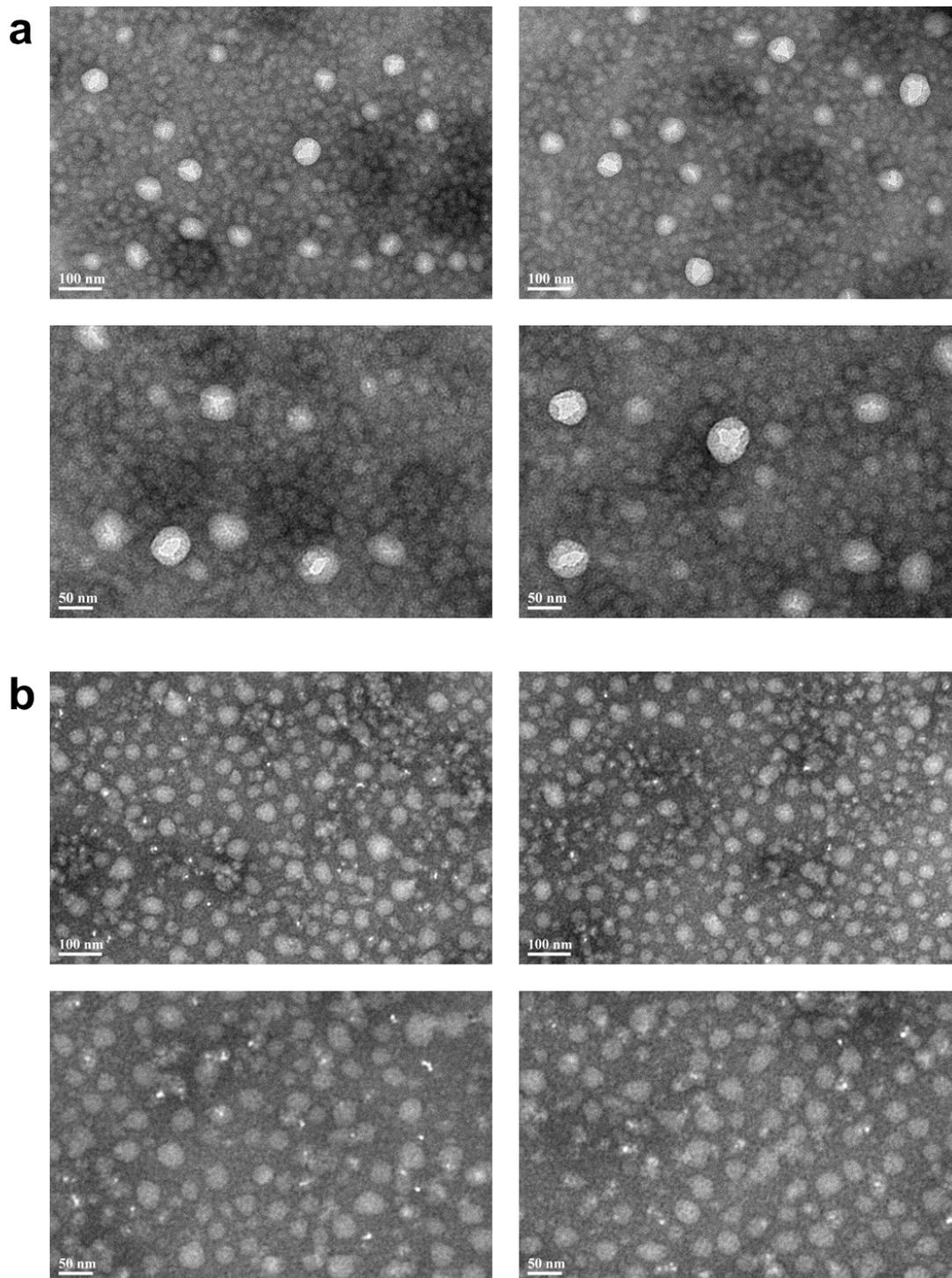
Figure S10. TEM images of NS-2 at different temperatures after negative staining with phosphotungstic acid. (a) 20 °C, (b) 60 °C.
