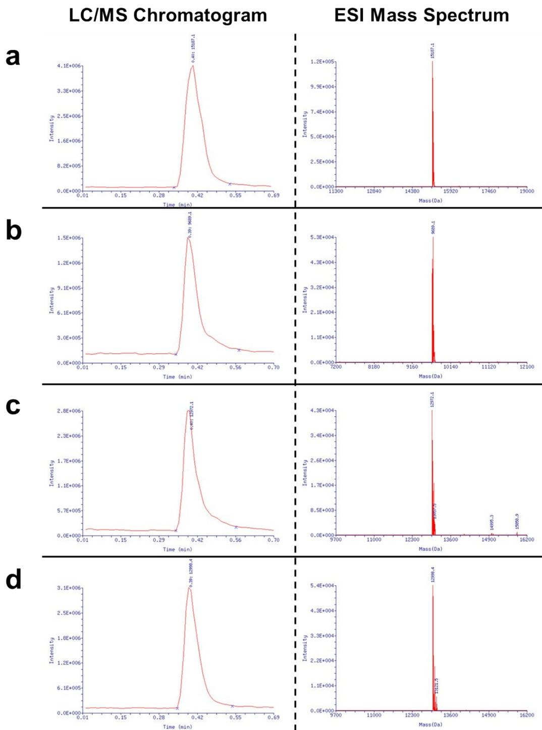
Figure S3. LC-MS data of ELP-ON conjugates. (a) ELP-ON1 (calculating mass: 15189.2, observed mass: 15187.1). (b) ELP-ON2 (calculating mass: 9668.8, observed mass: 9689.1). (c) ELP-ON3 (calculating mass: 12973.8, observed mass: 12972.1). (d) ELP-ON4 (calculating mass: 12997.8, observed mass: 12998.4).
