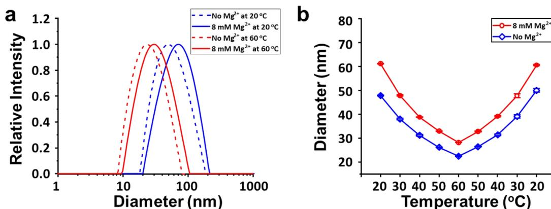
Figure S14. Temperature-dependent size regulation of NS-1 in 8 mM Mg<sup>2+</sup> or no Mg<sup>2+</sup>. (a) DLS characterization of NS-1 at two selected temperatures: 20 °C and 60 °C separately; (b) Analysis of hydrodynamic diameter of NS-1 as a function of temperature upon heating from 20 °C to 60 °C and then gradually decreasing from 60 °C back to 20 °C. Error bars were generated as the standard error of the mean from at least three replicates.
