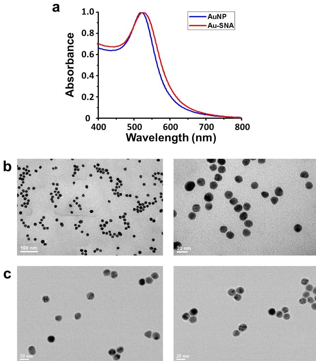
Figure S16. Characterization of AuNP and Au-SNA. (a) UV-Vis absorption spectrum of AuNP and Au-SNA. TEM images of (b) AuNP, (c) Au-SNA. Au-SNA sample was negative stained with uranyl acetat.
