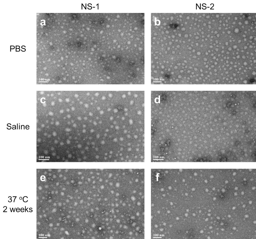
Figure S8. Stability analysis of NSs confirmed by TEM imaging. (a) NS-1 in PBS solution, (b) NS-2 in PBS solution, (c) NS-1 in physiological saline solution, (d) NS-2 in physiological saline solution, (e) NS-1 at 37 °C for 2 weeks, (f) NS-2 at 37 °C for 2 weeks.
