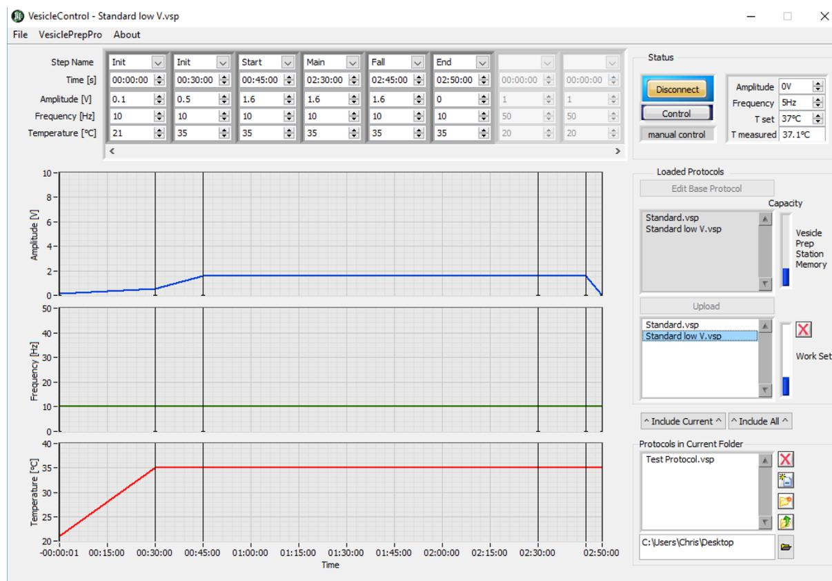
**Figure S7.** Electroformation protocol parameters displayed on the Nanion Vesicle Prep Pro *VesicleControl* software.
