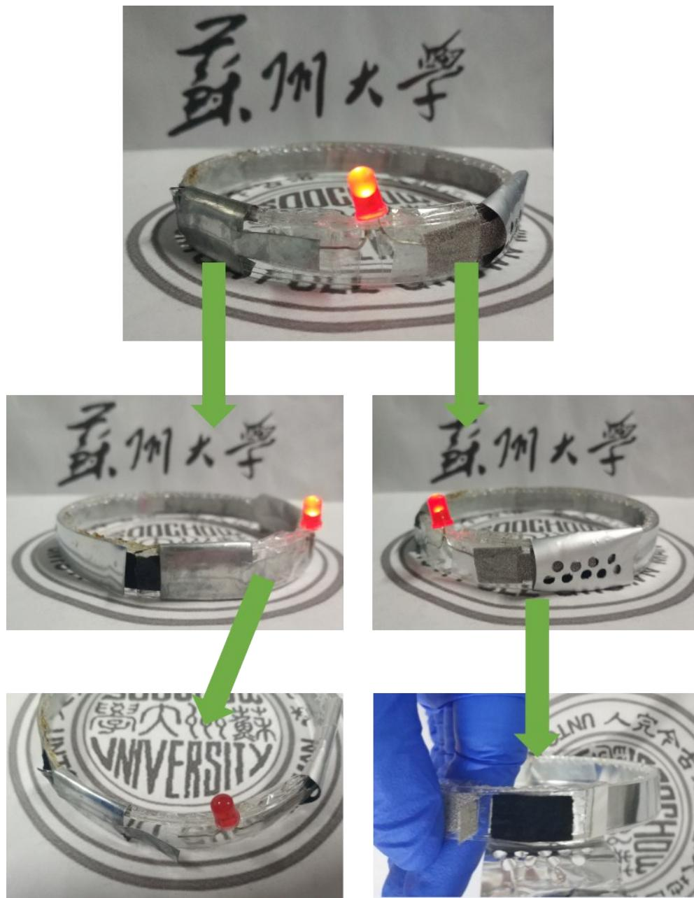
**Fig. S11.** Photograph of wearable device powered by two flexible Zn-air batteries with the NO-G@CP-2 as the air cathode connected in series.
