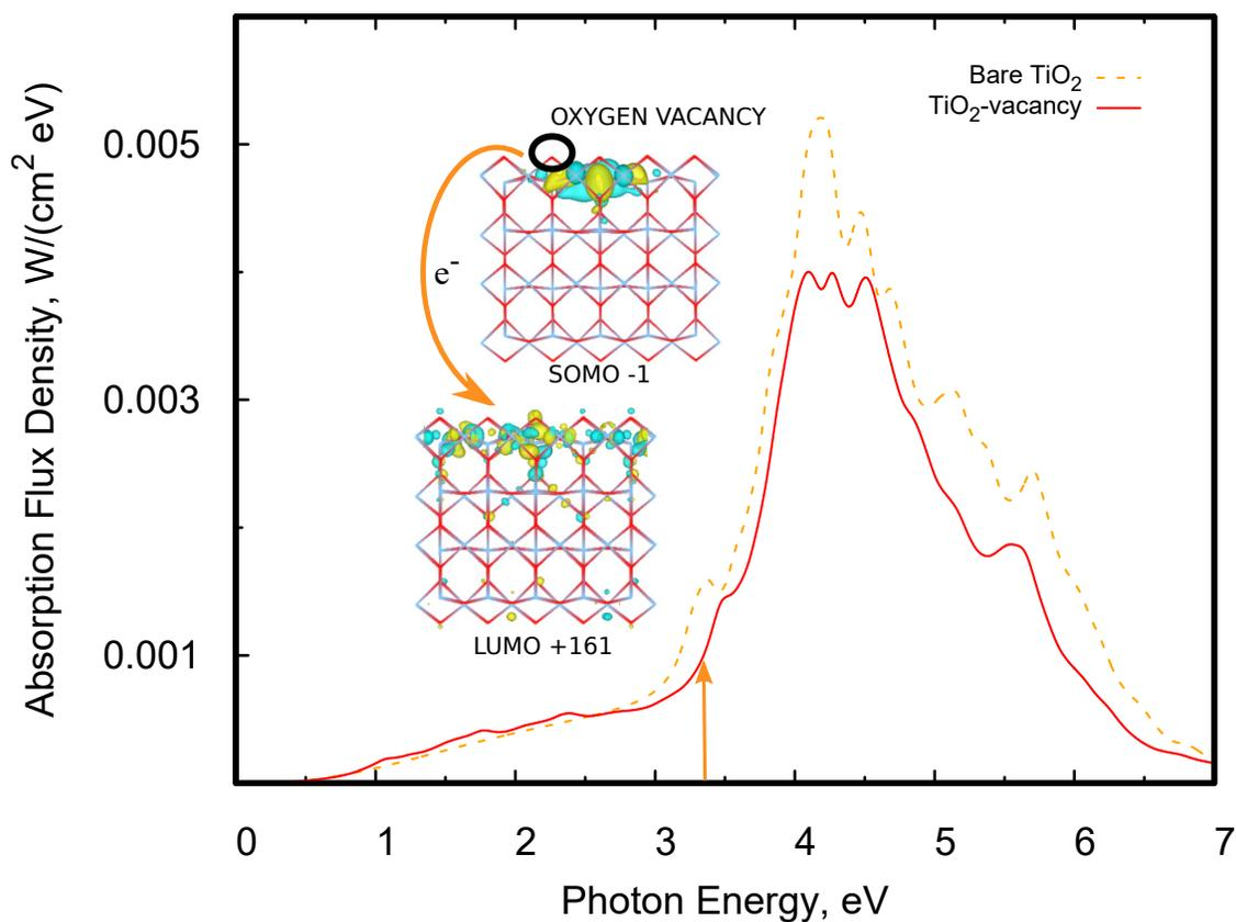
Figure S1: Upper panel: Electronic density of states (EDOS) of the reduced  $\text{TiO}_2(110)$  surface when bearing an oxygen vacancy. The SOMO and SOMO-1 orbitals are associated with the polaronic  $\text{Ti}^{3+} 3d^1$  states. Bottom panel: photo-absorption spectra of the same system. The insets present iso-density surfaces of the orbitals involved in the photo-induced transition from the surface polaronic states.
