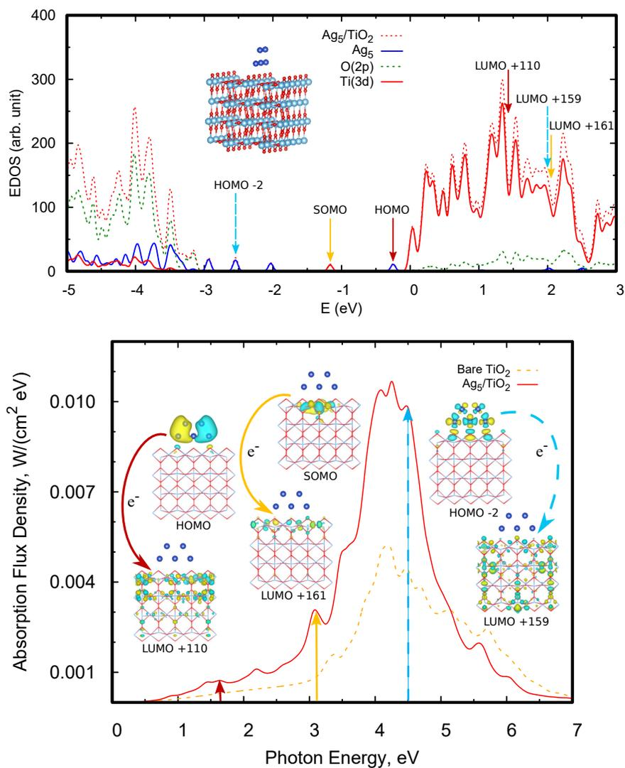
Figure S4: Same representation as in Figure 4 of the main manuscript but considering the  $\text{Ag}_5$  trapezoidal-shaped isomer. Upper panel: Electronic density of states (EDOS). Bottom panel: UV-Vis absorption spectra.
