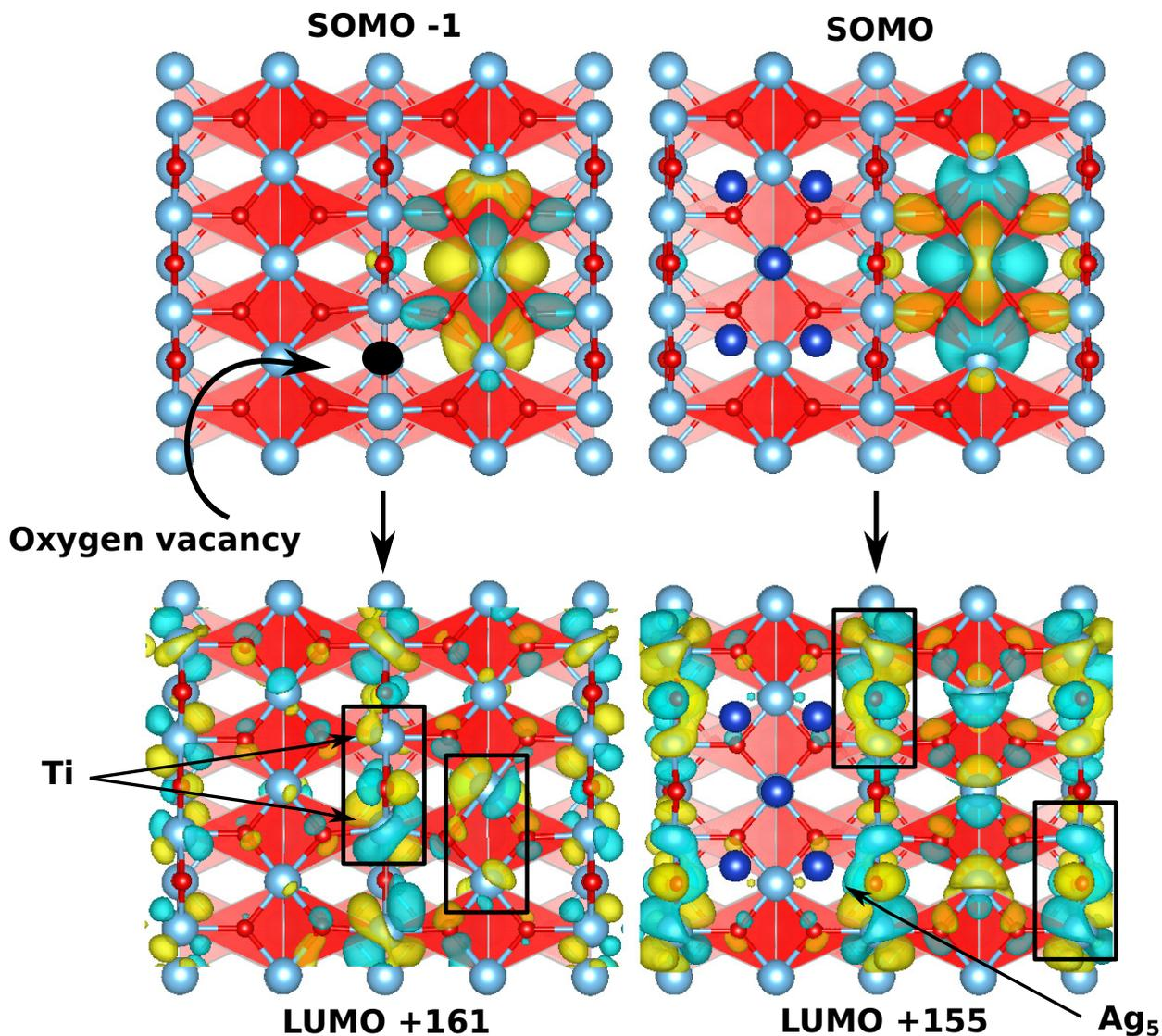
Figure S2: Top view of  $\text{TiO}_2$  surfaces bearing an oxygen vacancy (left-hand panels) and the  $\text{Ag}_5$  cluster (right-hand panels). The panels show the initial and final orbitals involved in the photo-excitation of the polaronic  $\text{Ti}^{3+} 3d^1$  states with sunlight. Notice that the electron-acceptor orbital shows a larger overlapping between atomic  $\text{Ti}(3d)$  orbitals when the surface polaron is induced through the  $\text{Ag}_5$  cluster deposition.
