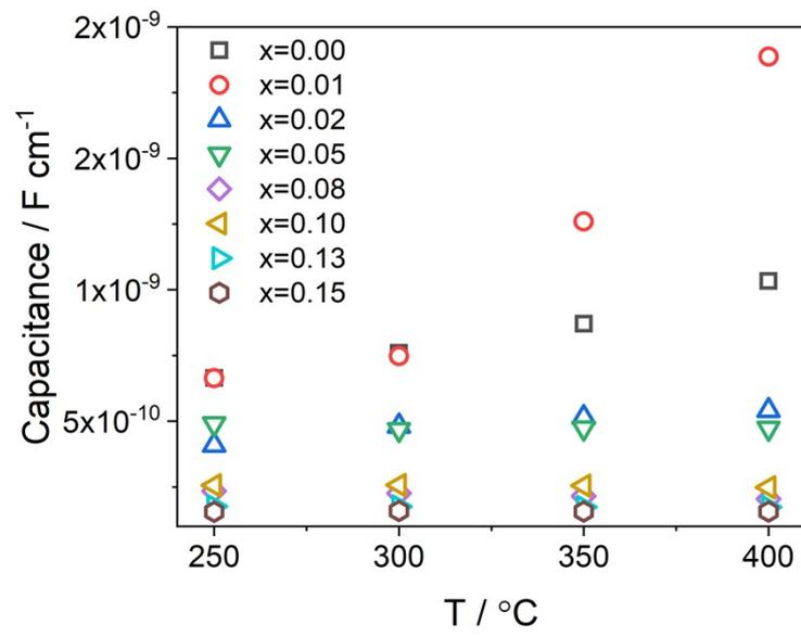
Figure S12. Variation in capacitance associated with the dominant  $M''$  peak in the  $M''$  spectra for BF-BT-xBLN ceramics in the temperature range  $\sim 250$  to  $400$   $^\circ\text{C}$ .
