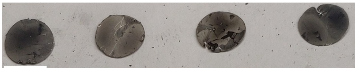
Fig. S30. Photographic snapshots of multiple PCNF-800 electrodes indicating successful melt infiltration of Na. Scale bar = 10 mm.
