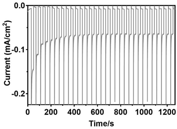
**Figure S5.** The *I-t* curve of ZnO/Cu<sub>2</sub>O photoelectrode at -0.2 V vs. Ag/AgCl (1 M KCl) in 0.1 M Na<sub>2</sub>SO<sub>4</sub> solution under visible-light irradiation (>420 nm)
