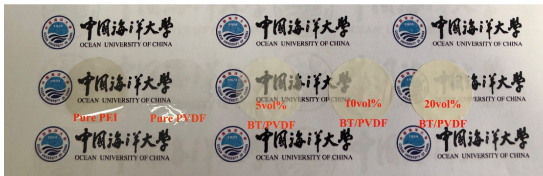
Fig. S2. Photograph of the single-layer films with different volume fractions of BaTiO 3 .
