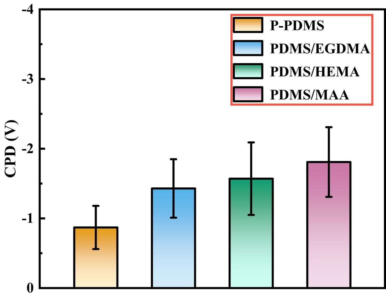
**Fig. S4** Summarized CPD results presented that the DN-PDMS was apt to attract an even greater amount of charge than P-PDMS.
