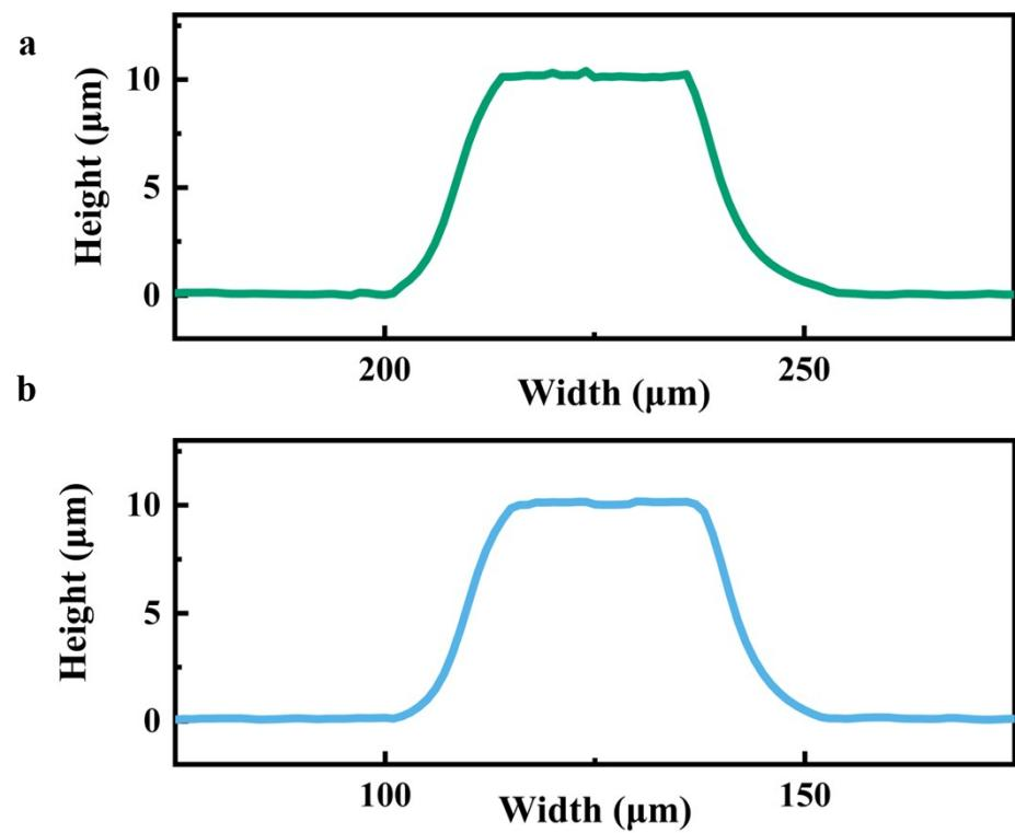
**Fig. S6** Surface profilometry depth profile for a section of a micro-patterned DN-PDMA with (a) lines and (b) cubes.
