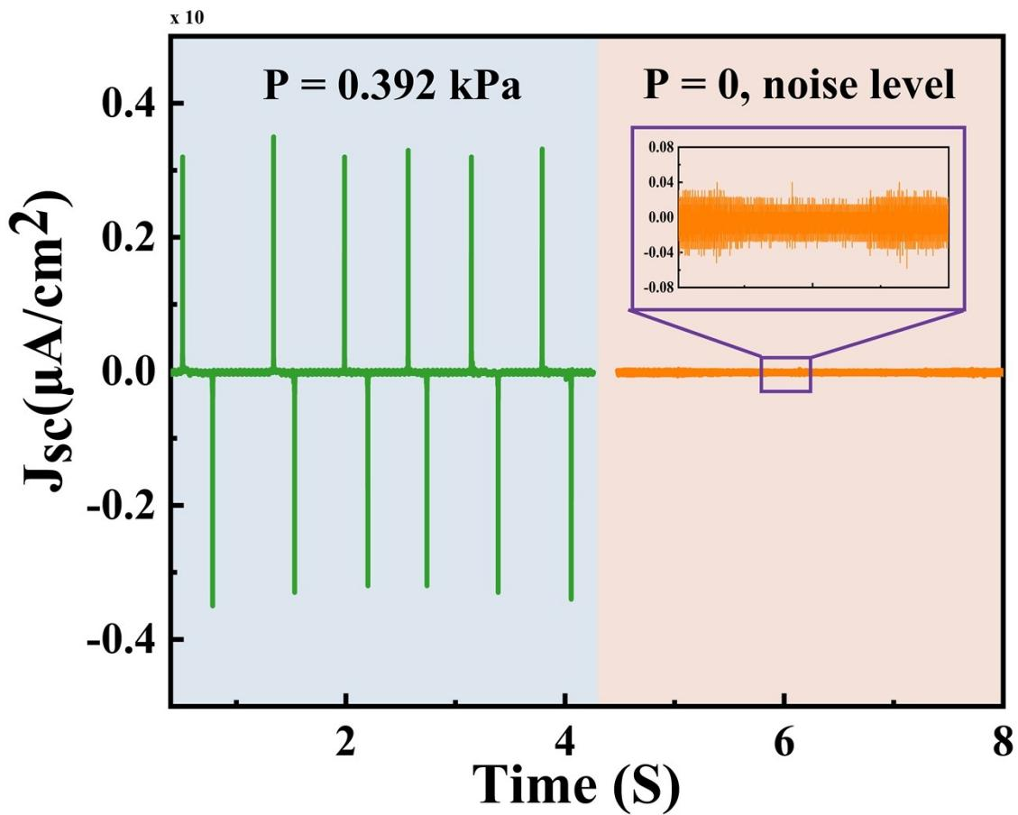
**Fig. S12** The measurement of the detection limit of the TENG through the short-circuit current density ( $J_{sc}$ ). The left panel in the plot shows the output  $J_{sc}$  with a gentle pressure applied on the TENG, while the right panel shows the measurement of the noise level magnitude. The inset is the enlarged view of the  $J_{sc}$  for the noise level with no pressure on. With this measurement the detection limit of the TENG could be deducted with the following equation.<sup>1</sup>
