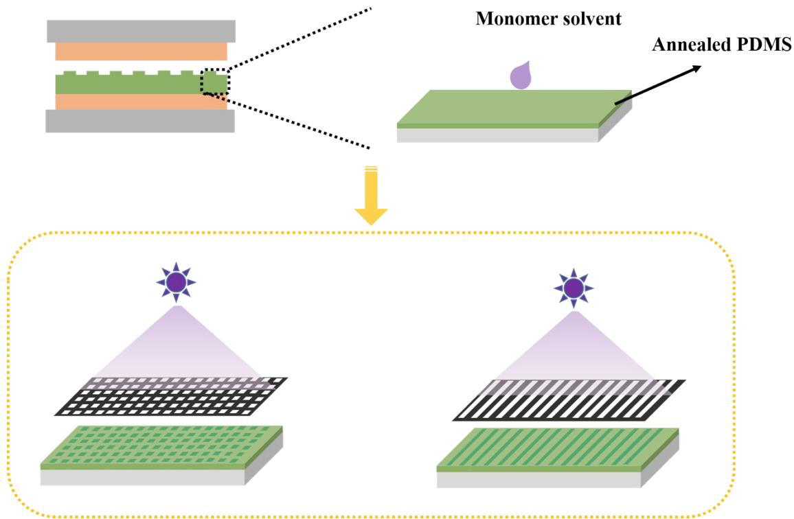
**Fig. S5** Schematic illustration of fabrication micro-patterned DN-PDMS layers.
