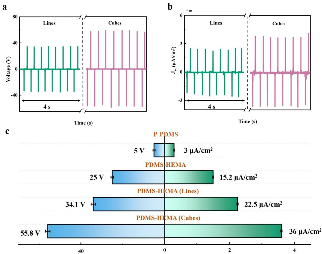
**Fig. S9** (a)  $V_{oc}$  and (b)  $J_{sc}$  of TENG with different patterned HEMA DN-PDMS films. (c) Summarized
