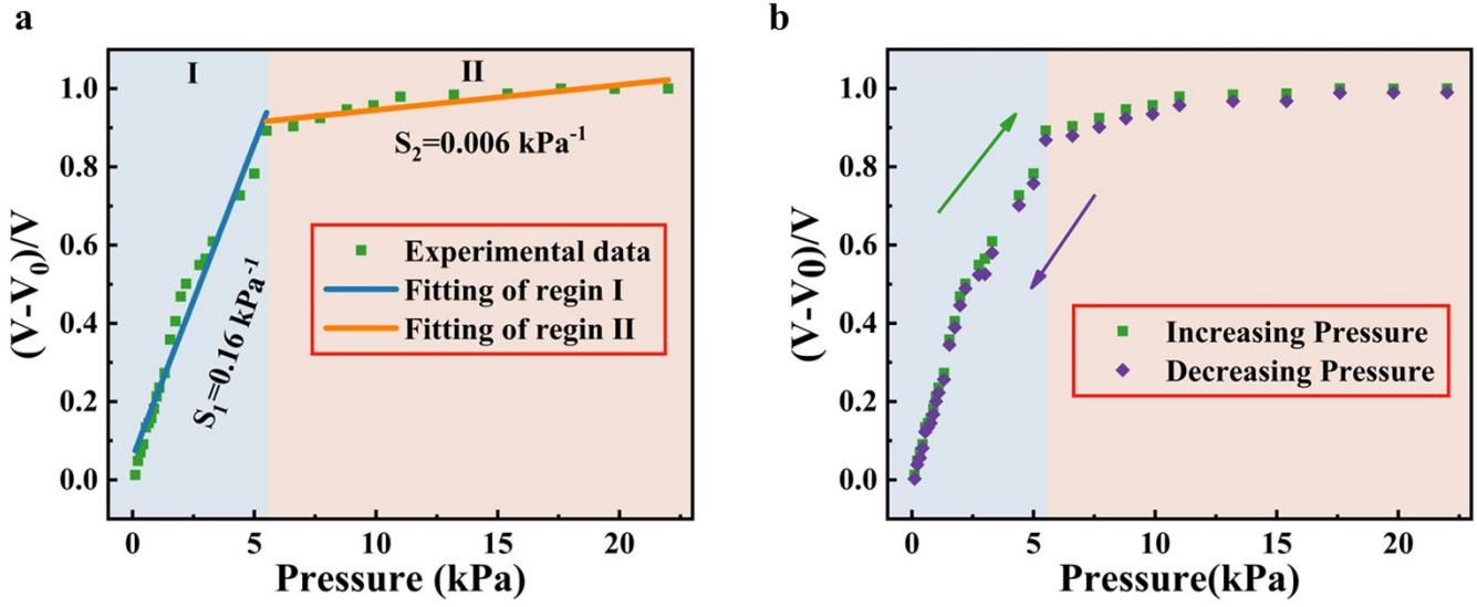
**Fig. S11** (a) Sensitivity of the TENG. (b) Hysteresis curve of the TENG.
