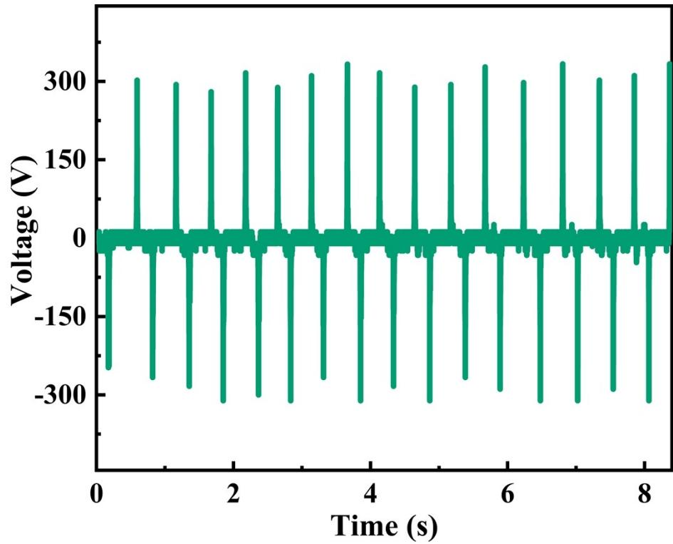
**Fig. S7**  $V_{oc}$  of cube DN-PDMS TENG with the size of  $2\text{ cm} \times 2\text{ cm}$ .
