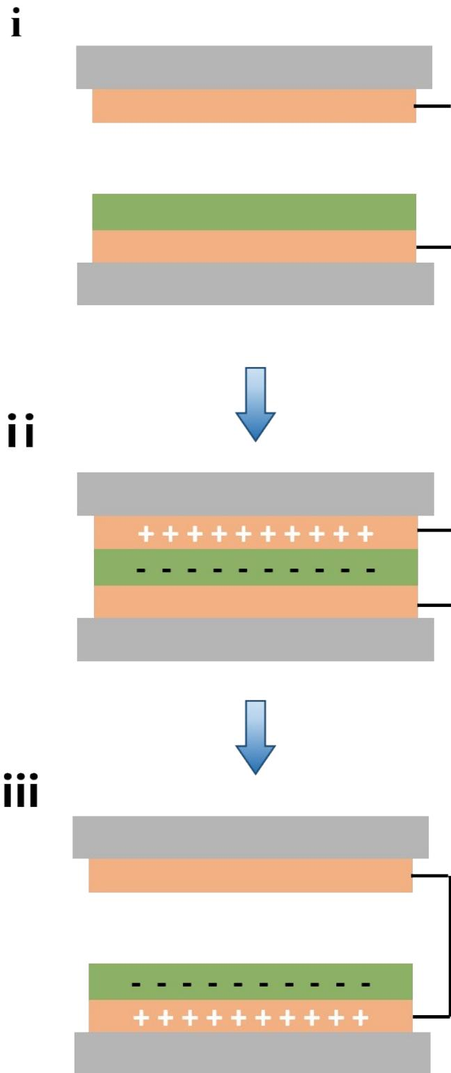
**Fig. S3** Working mechanism of original state TENG.
