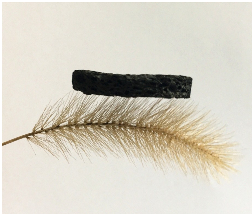
Fig. S4 Photograph of SnO 2 -SPM on a fragile setaria viridis , showing the ultralight performance of the synthesized SnO 2 -SPM.
