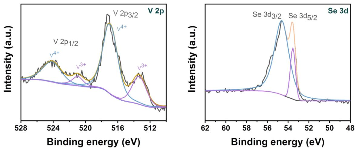
**Figure S1.** (a) High-resolution V 2p and (b) Se 3d XPS spectrum of VSe<sub>2</sub>.
