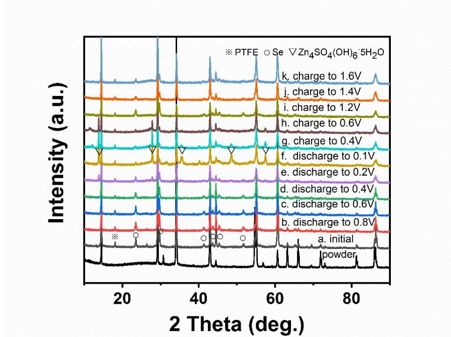
**Figure S5.** Ex situ XRD patterns at different charge/discharge states, in which the diffraction peaks of Se and  $\text{Zn}_4\text{SO}_4(\text{OH})_6 \cdot 5\text{H}_2\text{O}$  can be clearly observed.
