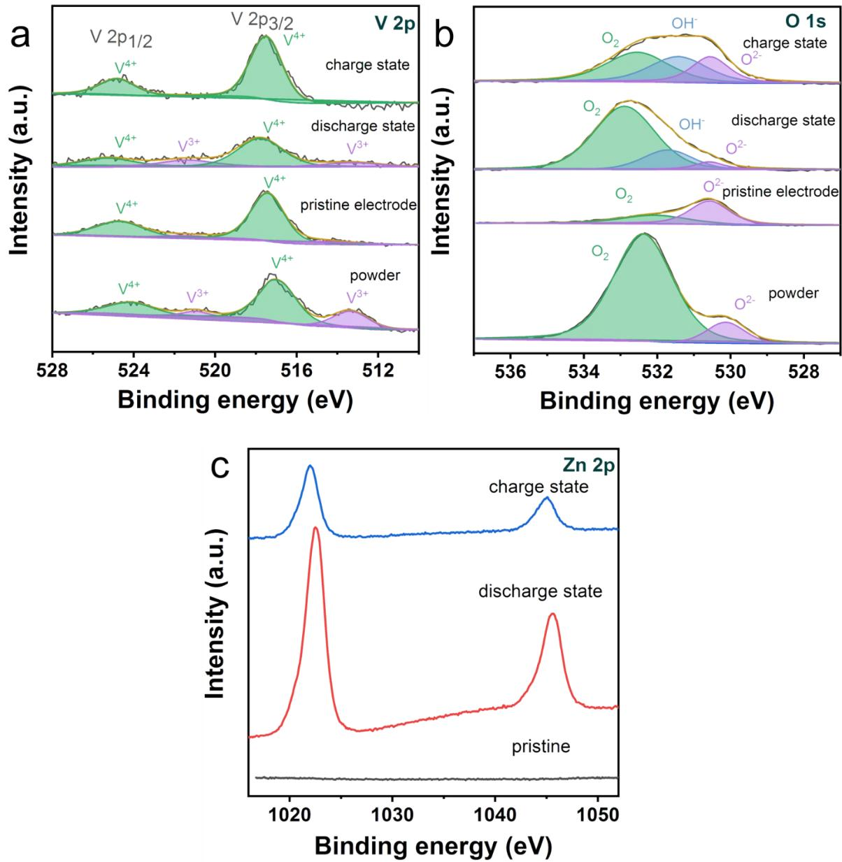
**Figure S7.** (a) V 2p, (b) O 1s and (c) Zn 2p XPS spectra in different states of VSe<sub>2</sub>.
