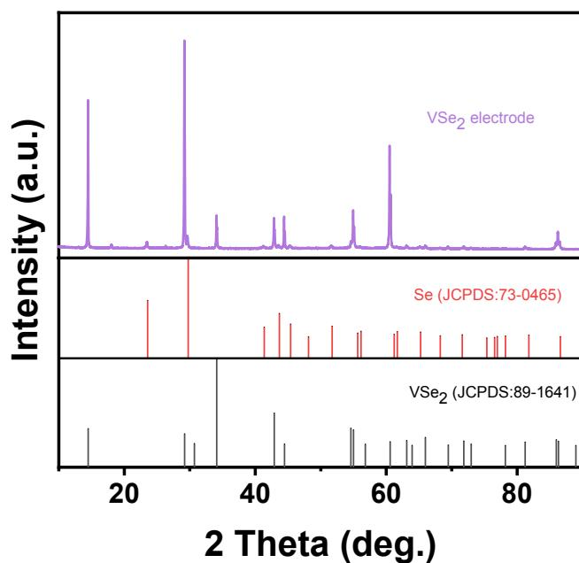
**Figure S2.** The XRD pattern of VSe<sub>2</sub> electrode after electrode fabrication.
