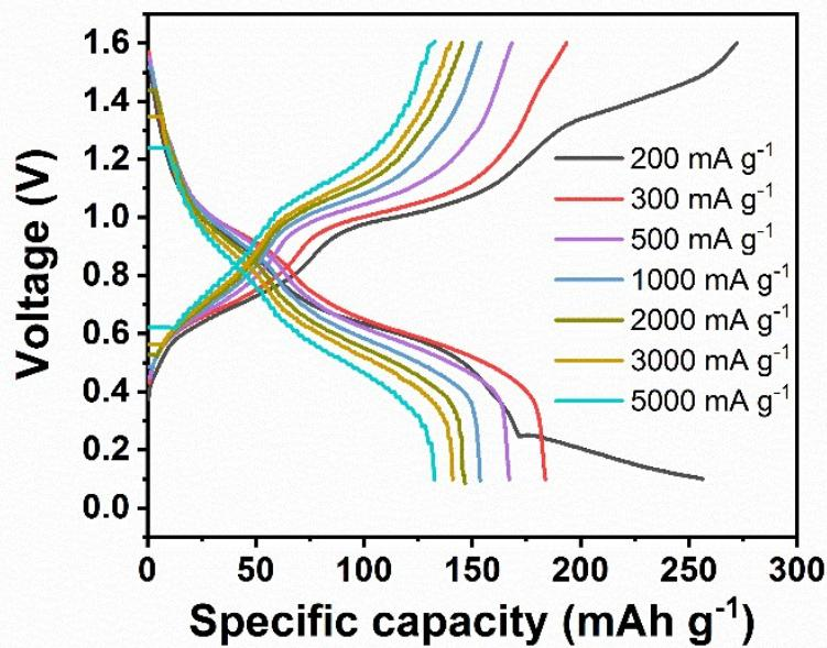
**Figure S4.** The charge/discharge profiles of Zn/VSe<sub>2</sub> battery at different current densities.
