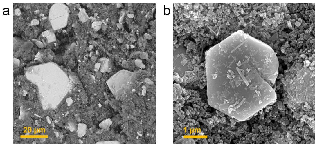
**Figure S3.** The SEM images of VSe<sub>2</sub> electrode material after electrode fabrication.
