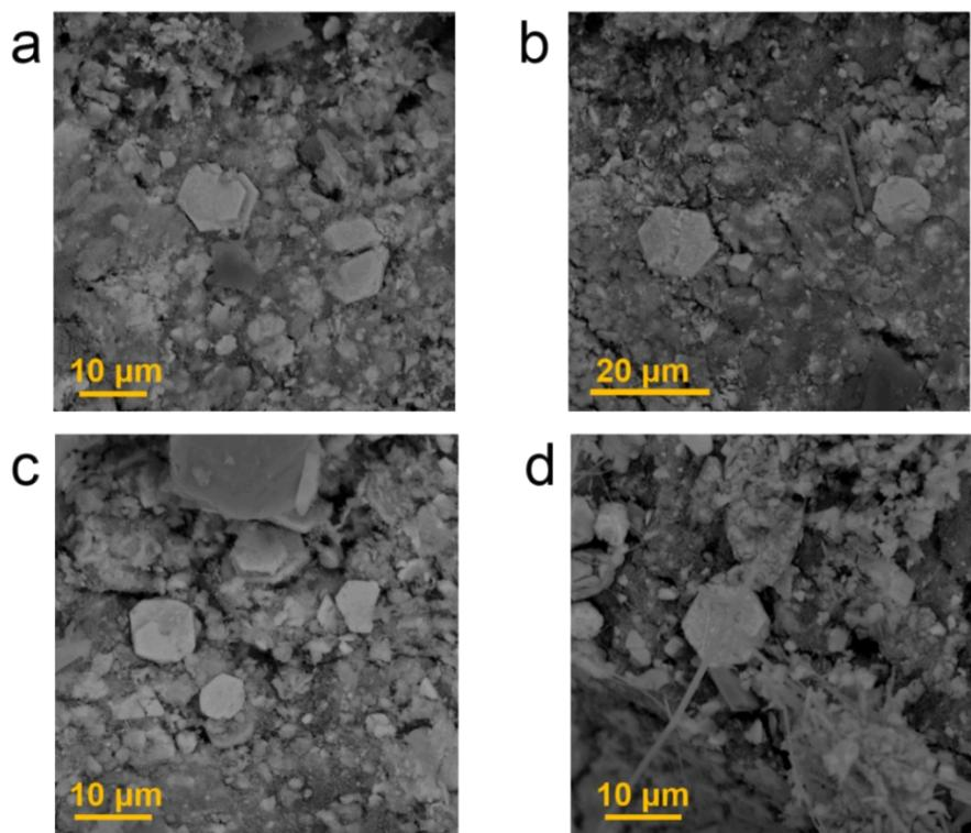
**Figure S6.** The SEM images of VSe<sub>2</sub> electrodes (a-b) after 20 cycles (c-d) and 50 cycles.
