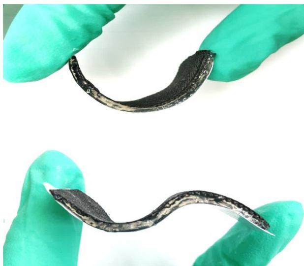
**Fig. S23.** Photos of the solid-state Zn-CO<sub>2</sub> electrochemical cells.
