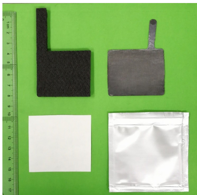
Figure S13. Exhibition of the components for the pouch battery. The pouch battery consists of one piece of carbon felt ( 40 \times 50 \times 5 mm) as cathode current collector, one piece of \text{PbSO}_4 anode ( 40 \times 50 mm) and a filter paper is used as separator.
