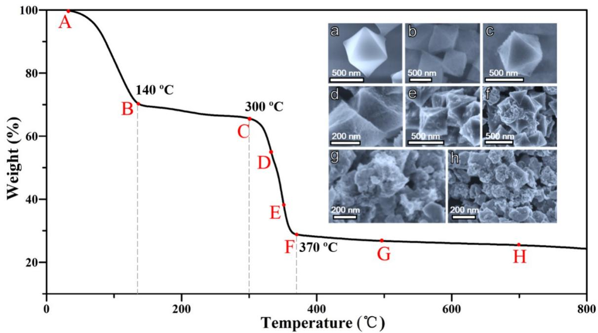
**Fig. S1** TGA plots for Cu-BTC, the insets a-g correspond to the SEM images of A-G in TGA, respectively.
