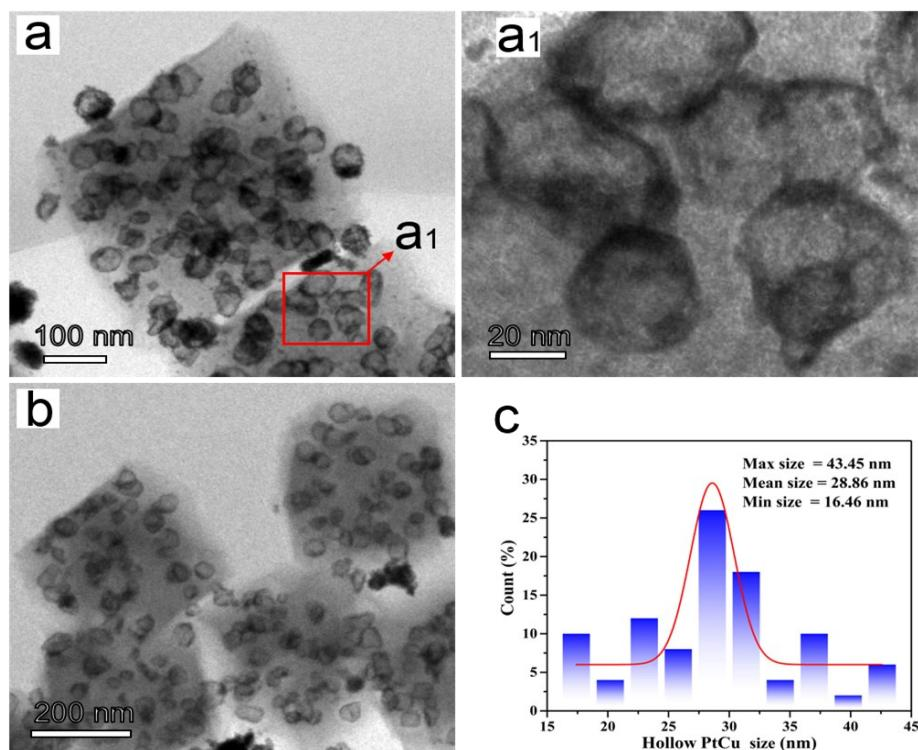
**Fig. S3** (a-b) TEM images of S-H-Pt<sub>x</sub>Cu<sub>y</sub>@C. (a<sub>1</sub>) Enlarged TEM image of selected area labelled in (a). (c) The diameter distribution histograms of spherical hollow PtCu alloy statistics from (b).
