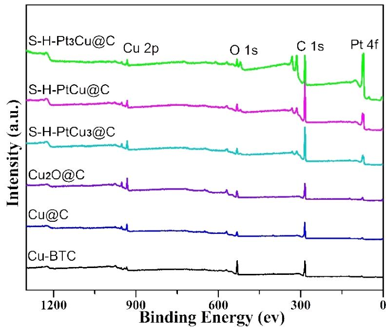
**Fig. S5** Full range XPS spectrum of Cu-BTC, Cu@C, Cu<sub>2</sub>O@C and S-H-Pt<sub>x</sub>Cu<sub>y</sub>@C.
