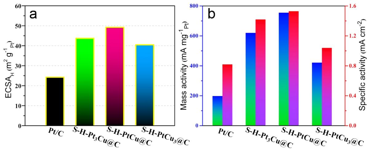
**Fig. S7** (a) The electrochemically active surface area of S-H-Pt<sub>x</sub>Cu<sub>y</sub>@C and commercial Pt/C catalysts. (b) Mass activity and Specific activity of S-H-Pt<sub>x</sub>Cu<sub>y</sub>@C and commercial Pt/C catalysts
