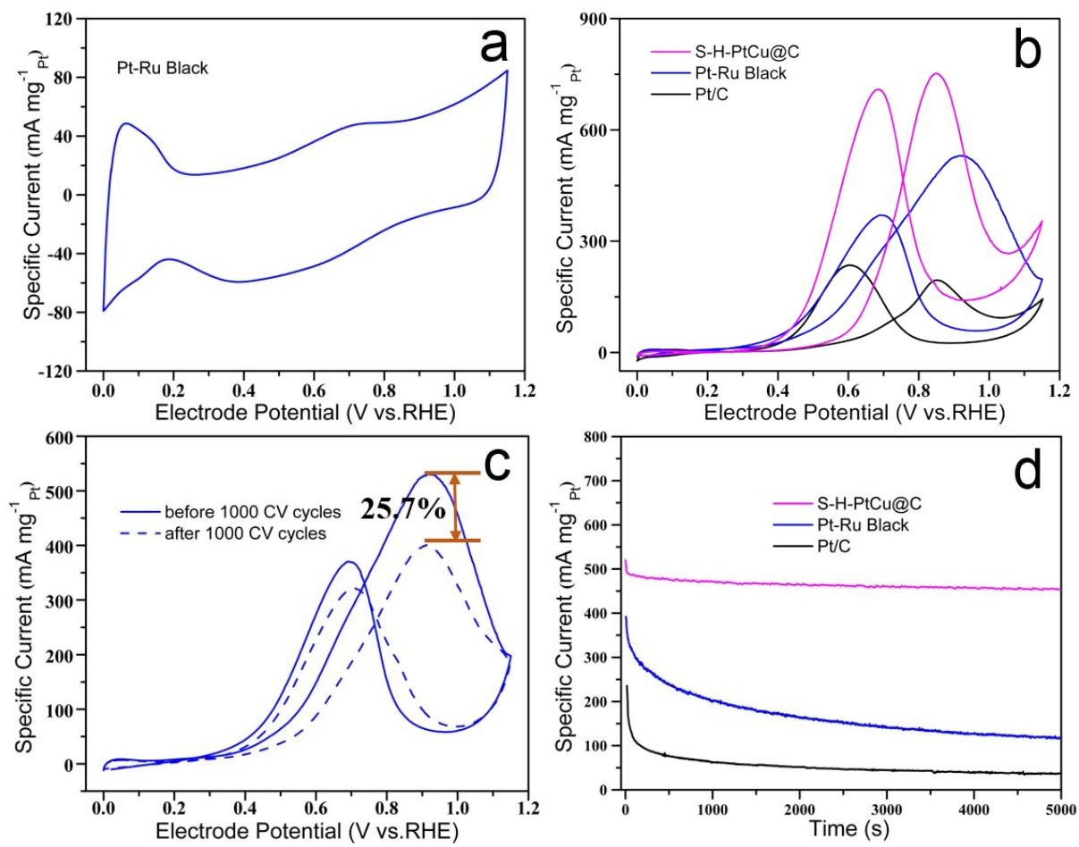
**Fig. S12** (a) CV curves of S-H-PtCu@C, commercial Pt-Ru Black and commercial PtRu catalysts in 0.5 M  $\text{H}_2\text{SO}_4$ . (b) CV curves of S-H-PtCu@C, commercial Pt-Ru Black and commercial PtRu catalysts in 0.5 M  $\text{H}_2\text{SO}_4$  + 1 M methanol. (c) CV curves of commercial Pt-Ru Black before and after 1000 potential cycles. (d) Chronoamperometric measurements.
