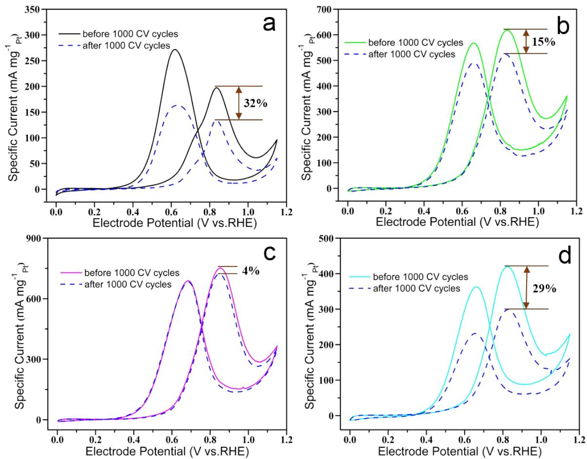
**Fig. S9 (a-d)** CV curves of commercial Pt/C, S-H-Pt<sub>3</sub>Cu@C, S-H-PtCu@C and S-H-PtCu<sub>3</sub>@C catalysts before and after 1000 potential cycles.
