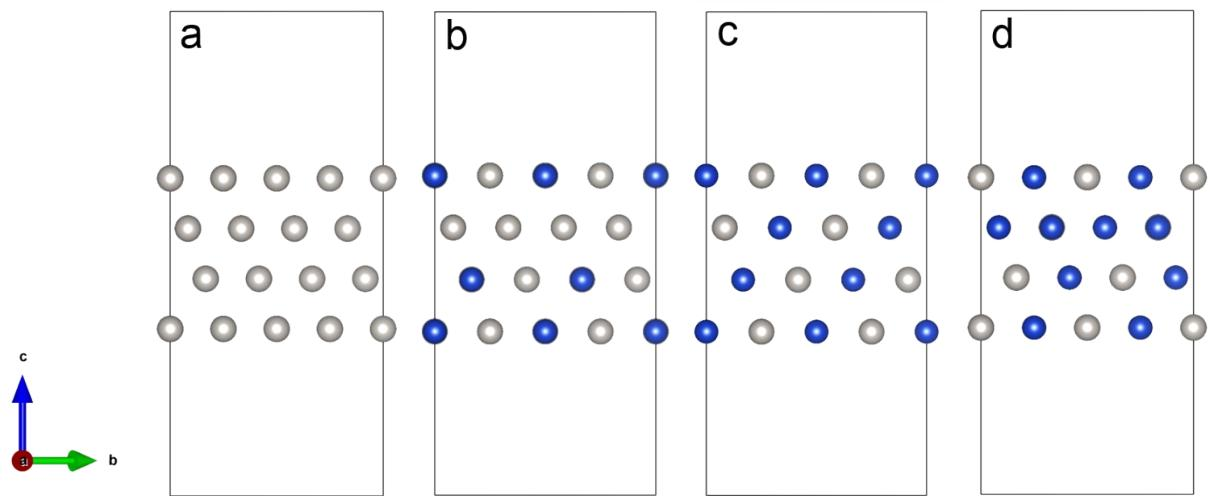
**Fig. S14 (a-d)** Structural models of  $\text{Pt}(111)$ ,  $\text{Pt}_3\text{Cu}(111)$ ,  $\text{PtCu}(111)$  and  $\text{PtCu}_3(111)$  slabs.
