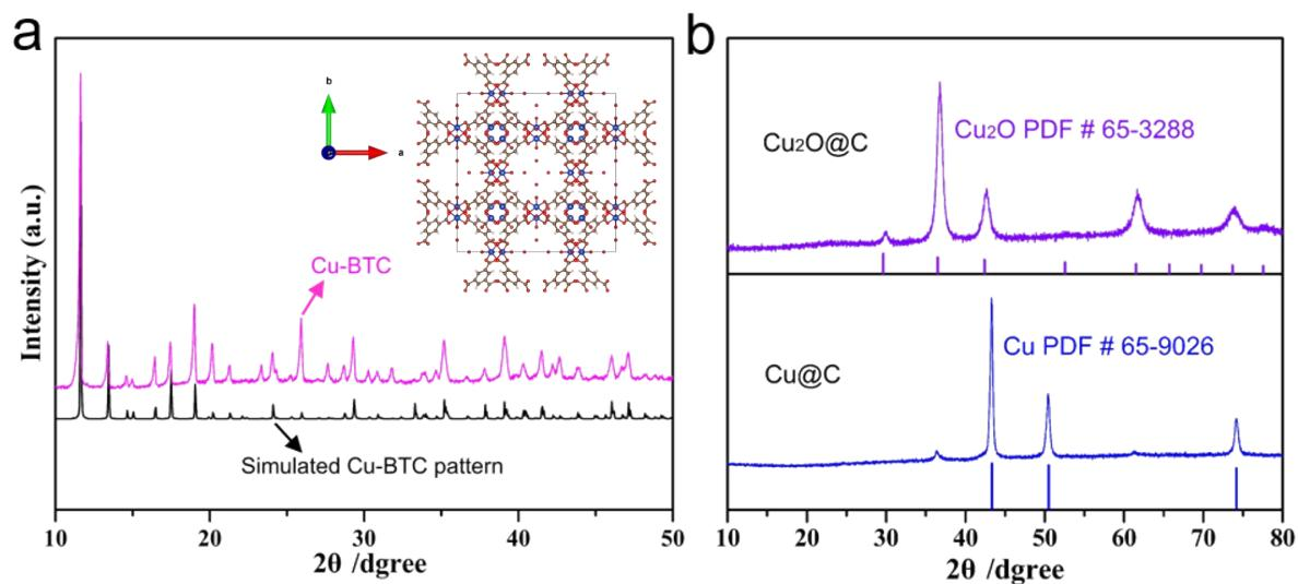
**Fig. S2** (a) XRD patterns of Cu-BTC and the simulated XRD pattern of Cu-BTC by Materials Studio 7.0, the insets show the crystal structure of Cu-BTC (blue, gray, red and pink spheres represent Cu, C, O and H atoms, respectively). (b) XRD patterns of Cu@C and Cu<sub>2</sub>O@C.
