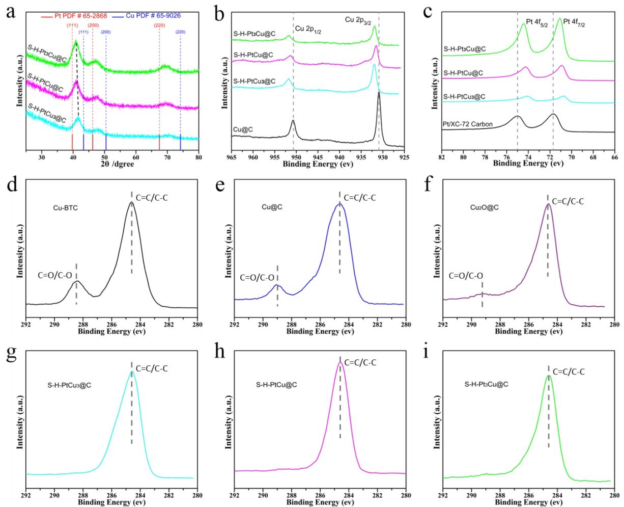
**Fig. S4** (a) XRD pattern of S-H-Pt<sub>x</sub>Cu<sub>y</sub>@C. (b) Cu 2p XPS spectra of S-H-Pt<sub>x</sub>Cu<sub>y</sub>@C and Cu@C. (c) Pt 4f XPS spectra of S-H-Pt<sub>x</sub>Cu<sub>y</sub>@C and Pt/XC-72 Carbon. (d-i) C 1s XPS spectra of Cu-BTC, Cu@C, Cu<sub>2</sub>O@C, S-H-PtCu<sub>3</sub>@C, S-H-PtCu@C and S-H-Pt<sub>3</sub>Cu@C.
