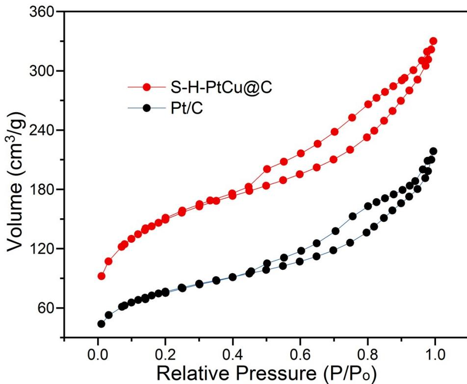
**Fig. S8** Nitrogen adsorption and desorption isotherms of S-H-PtCu@C and commercial Pt/C.
