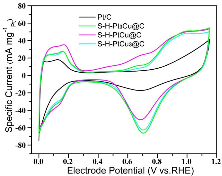
**Fig. S6** CV curves of S-H-Pt<sub>x</sub>Cu<sub>y</sub>@C and commercial Pt/C catalysts in 0.5 M H<sub>2</sub>SO<sub>4</sub>.
