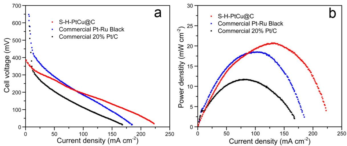
**Fig. S13** (a) Polarization curves and (b) power density of S-H-PtCu@C, commercial Pt-Ru Black and commercial 20% Pt/C in DMFCs.
