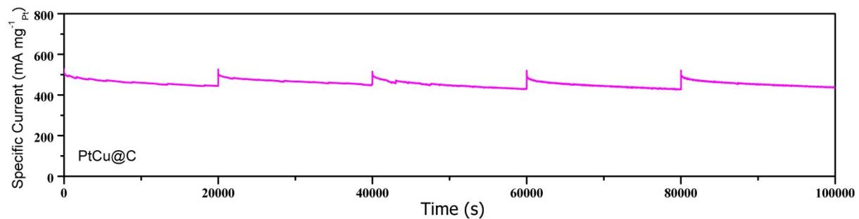
**Fig. S10** Long-term durability measurements of S-H-PtCu@C catalyst, the arrows indicate when electrocatalysts were reactivated in clean 0.5 M  $\text{H}_2\text{SO}_4$ .
