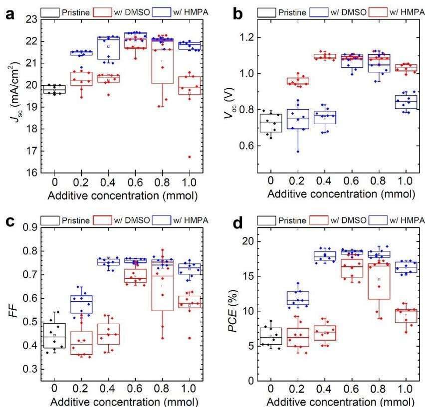
**Figure S3.** Statistical photovoltaic parameters depending on Lewis base additive concentration. (a) Short-circuit photocurrent density ( $J_{sc}$ ), (b) open-circuit voltage ( $V_{oc}$ ), (c) fill factor ( $FF$ ), and (d) power conversion efficiency ( $PCE$ ).  $J$ - $V$  data were obtained under AM 1.5G simulated 1 sun illumination at a scan rate of 0.26 V/s. The active area was 0.125 cm<sup>2</sup>. Reverse scanned data are presented.
