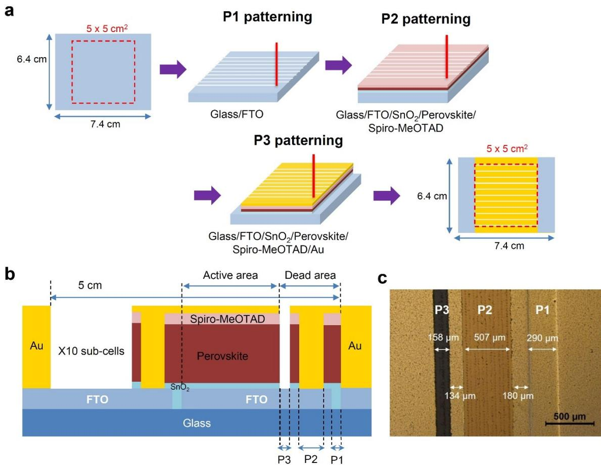
**Figure S4.** Schematic illustration of (a) the fabrication process and (b) the structure of the perovskite mini-module with 10 sub-cells connected in series. (c) Optical microscopic image of P1, P2, and P3 lines scribed on the mini-module.
