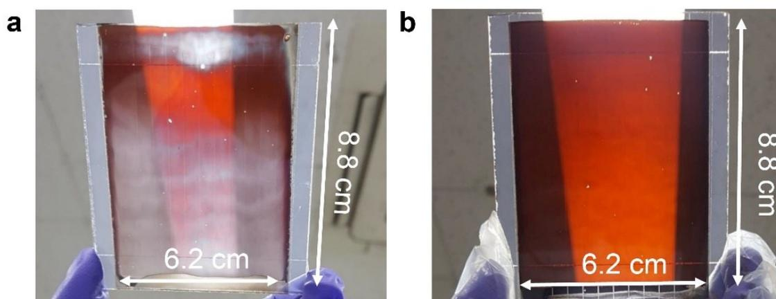
**Figure S1.** Digital photographs of the D-bar coated and 150 °C-annealed perovskite films formed from (a) the DMSO-contained and (b) the HMPA-contained precursor solution. The substrate size was 8.8 cm × 6.2 cm. FTO side was exposed (the perovskite films were faced on the backside fluorescent light).
