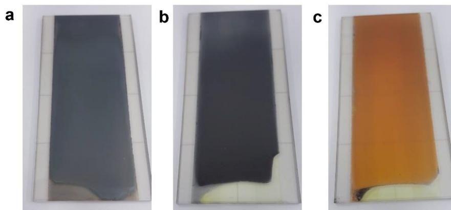
**Figure S2.** Digital photographs of the as-coated non-annealed films formed from the precursor solution (a) without Lewis base additive and with Lewis base additive of (b) DMSO or (c) HMPA.
