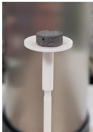
Figure A 8. Example of monolith used for TGA.
