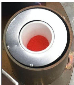
Figure S4. (a) Appearance of the remaining material in the crucible after the SSVD of \text{CsBi}_3\text{I}_{10} and (b) XRD diffractograms of the \text{CsBi}_3\text{I}_{10} in powder (starting material for the SSVD, green), the remaining powder in the crucible (pink), \text{Cs}_3\text{Bi}_2\text{I}_9 (possible decomposition product, grey) and \text{BiI}_3 (starting reagent of \text{CsBi}_3\text{I}_{10} , ICSD 56573, blue).
