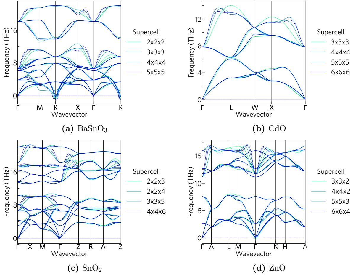
**Figure S4:** The convergence of the phonon band structure with supercell size, as in Figure S3, but without the non-analytical correction.<sup>6,7</sup>
