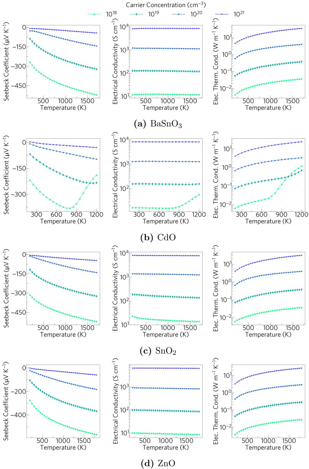
**Figure S2:** Plots of Seebeck coefficient, electrical conductivity, and electronic thermal conductivity, against temperature at various  $n$ -type carrier concentrations for (a) BaSnO<sub>3</sub>, (b) CdO, (c) SnO<sub>2</sub> and (d) ZnO. The values have been averaged across crystal orientation for SnO<sub>2</sub> and ZnO as real devices would need to be nanostructured.
