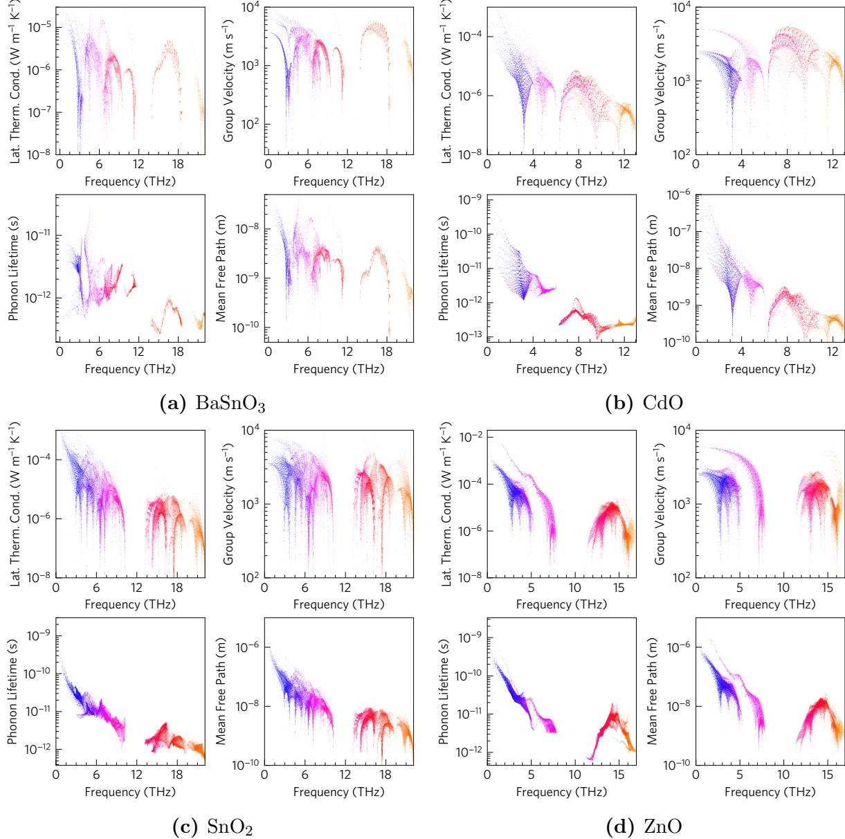
**Figure S5:** Clockwise from top left per subfigure, the lattice thermal conductivity, group velocity, mean free path and lifetime for each mode at each  $q$ -point, coloured by band, for (a) BaSnO<sub>3</sub>, (b) CdO, (c) SnO<sub>2</sub> and (d) ZnO. Data calculated with Phono3py.<sup>8</sup>
