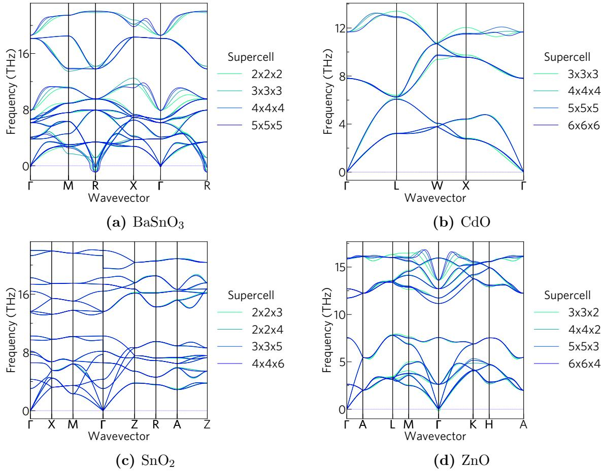
**Figure S3:** The convergence of the phonon band structure with supercell size, calculated with Phonopy,<sup>6</sup> including the non-analytical correction.<sup>7</sup>
