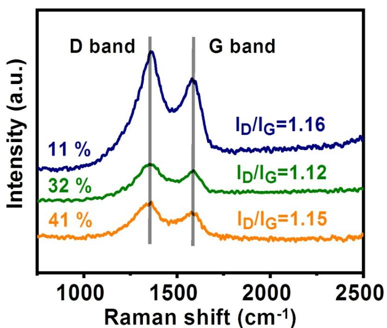
**Fig. S6** Raman spectra of Fe/Fe<sub>3</sub>C-NCNF-1 (iron content: 11%, pyrolysis at 500 °C), Fe/Fe<sub>3</sub>C-NCNF-2 (iron content: 32%, pyrolysis at 500 °C), Fe/Fe<sub>3</sub>C-NCNF-3 (iron content: 41%, pyrolysis at 500 °C).
