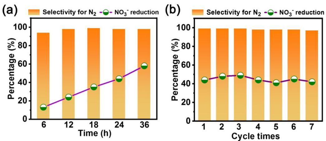
**Fig. S16** (a) Conversion percentage of nitrate and nitrogen selectivity of Fe/Fe<sub>3</sub>C-NCNF-2 (iron content: 32%, pyrolysis at 500 °C) at different reaction time, (b) conversion percentage of nitrate and nitrogen selectivity over 7 cycles test of electrocatalytic denitrification. Reaction conditions: initial  $\text{NO}_3^-$ -N concentration 100 mg/L, 0.03 M NaCl and 0.01 M  $\text{Na}_2\text{SO}_4$ , initial pH value 5 at 24 h.
