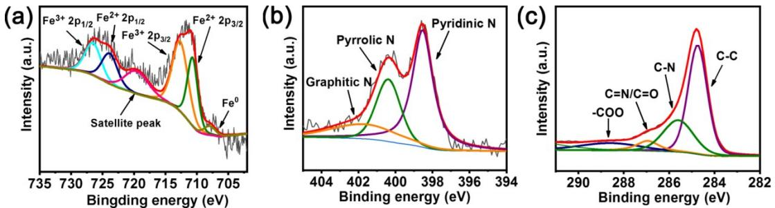
**Fig. S8** High resolution XPS spectra of (a) Fe 2p, (b) N 1s, and (c) C 1s of Fe/Fe<sub>3</sub>C-NCNF-2-600 (iron content: 32%, pyrolysis at 600 °C).
