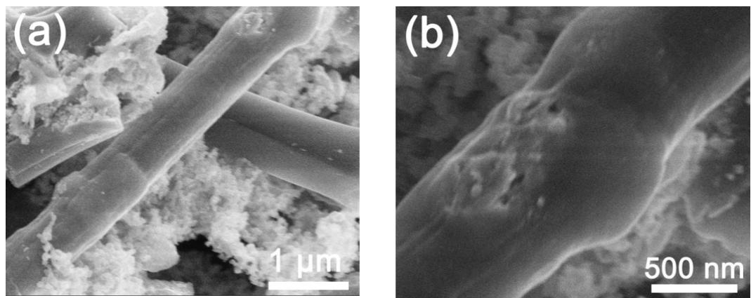
**Fig. S17** (a,b) SEM images of Fe/Fe<sub>3</sub>C-NCNF-2 after 7 cycles test of electrocatalytic denitrification of Fe/Fe<sub>3</sub>C-NCNF-2 (iron content: 32%, pyrolysis at 500 °C).
