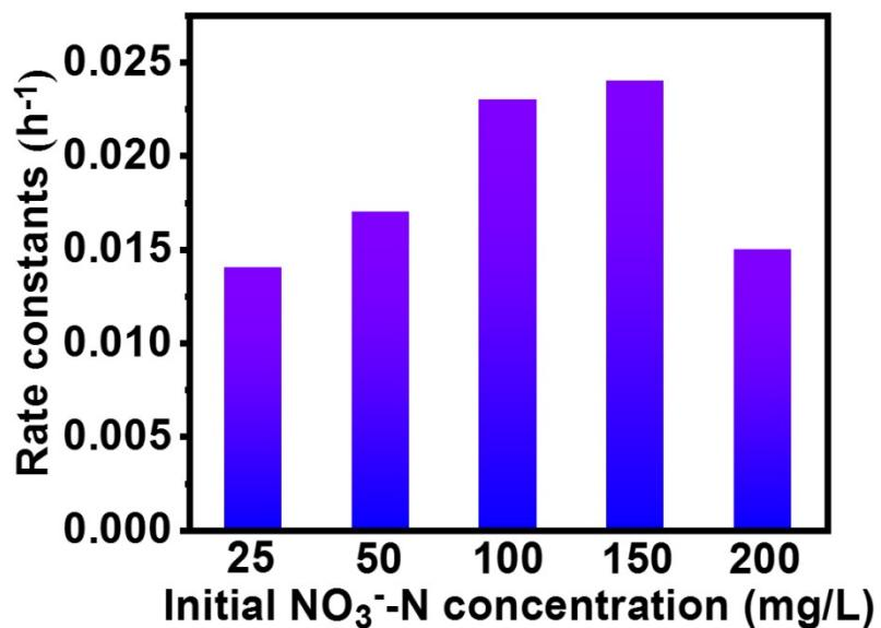
**Fig. S13** The rate constants of electrocatalytic denitrification of Fe/Fe<sub>3</sub>C-NCNF-2 (iron
