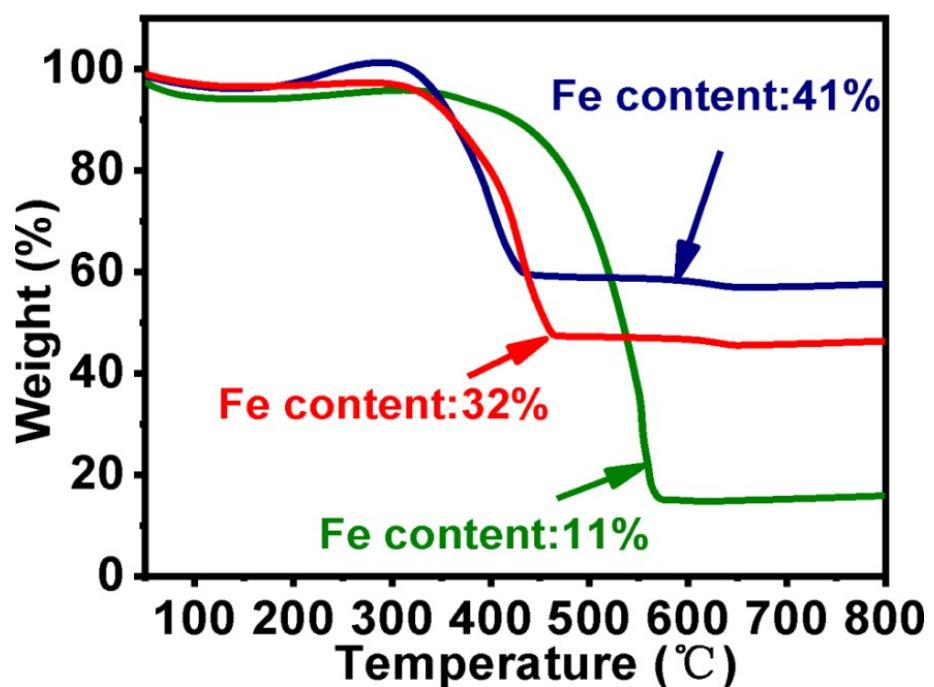
**Fig. S2** TGA curves of Fe/Fe<sub>3</sub>C-NCNF-1 (iron content: 11%, pyrolysis at 500 °C), Fe/Fe<sub>3</sub>C-NCNF-2 (iron content: 32%, pyrolysis at 500 °C), Fe/Fe<sub>3</sub>C-NCNF-3 (iron
