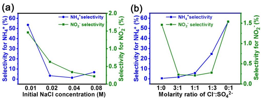
**Fig. S12** Effects of (a) initial Cl<sup>-</sup> concentration and (b) the molarity ratio of Cl<sup>-</sup> and SO<sub>4</sub><sup>2-</sup> on nitrite selectivity and ammonia selectivity of Fe/Fe<sub>3</sub>C-NCNF-2 (iron content: 32%, pyrolysis at 500 °C). Reaction conditions: initial NO<sub>3</sub><sup>-</sup>-N concentration 100 mg/L, initial pH value 5 at 24 h for (a), initial NO<sub>3</sub><sup>-</sup>-N concentration 100 mg/L, initial pH value 5 at 24 h for (b).
