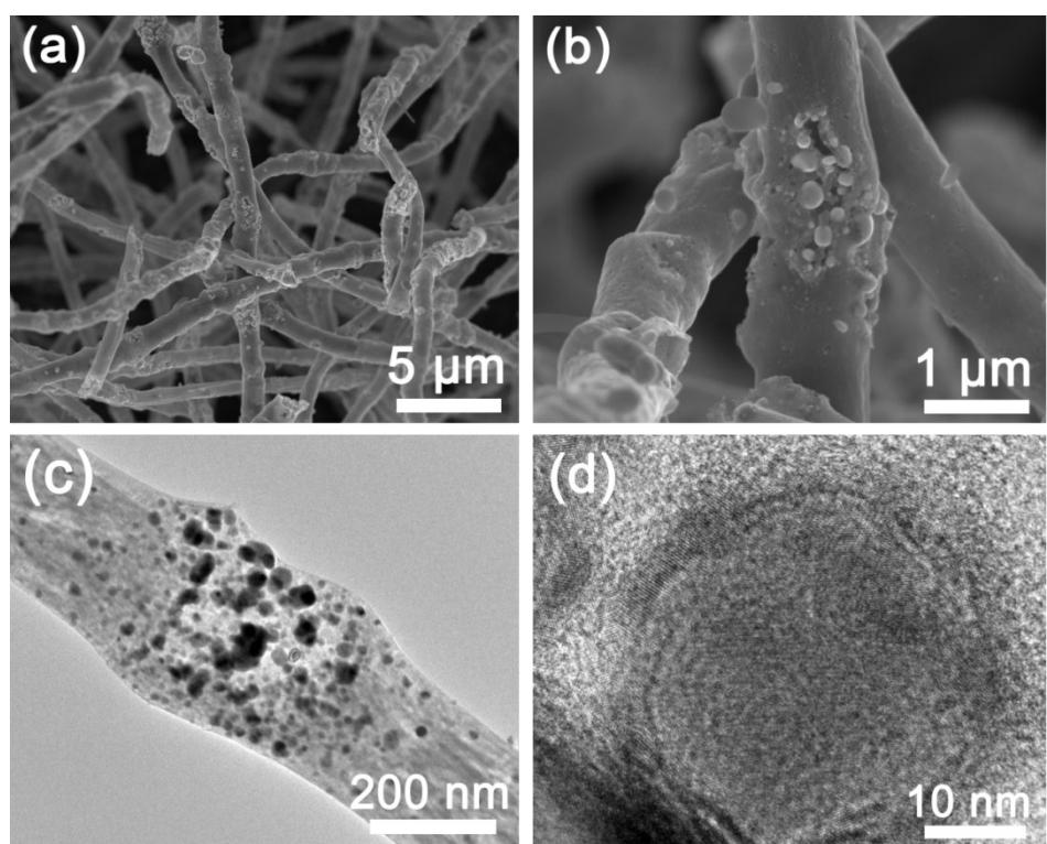
**Fig. S5** (a, b) SEM images, (c) TEM image, and (d) HRTEM image of Fe/Fe<sub>3</sub>C-NCNF-2-600 (iron content: 32%, pyrolysis at 600 °C).
