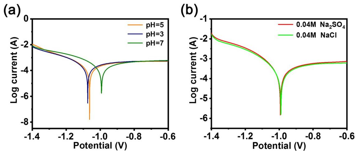
**Fig. S11** Potentiodynamic polarization curves of Fe/Fe<sub>3</sub>C-NCNF-2 (iron content: 32%, pyrolysis at 500 °C) at (a) different pH values and in (b) 0.04 M Na<sub>2</sub>SO<sub>4</sub>, 0.04 M NaCl electrolyte. Reaction conditions: initial NO<sub>3</sub><sup>-</sup>-N concentration 100 mg/L, 0.02 M NaCl for (a), initial NO<sub>3</sub><sup>-</sup>-N concentration 100 mg/L, 0.04 M NaCl and 0.04 M Na<sub>2</sub>SO<sub>4</sub>, initial pH value 5 for (b).
