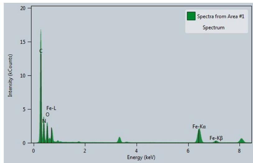
**Fig. S9** EDS spectrum of Fe/Fe<sub>3</sub>C-NCNF-2 (iron content: 32%, pyrolysis at 500 °C).
