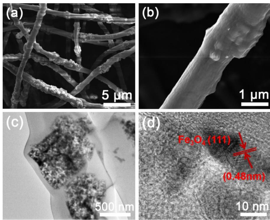
**Fig. S4** (a, b) SEM images, (c) TEM image, and (d) HRTEM image of Fe/Fe<sub>3</sub>C-NCNF-2-400 (iron content: 32%, pyrolysis at 400 °C).
