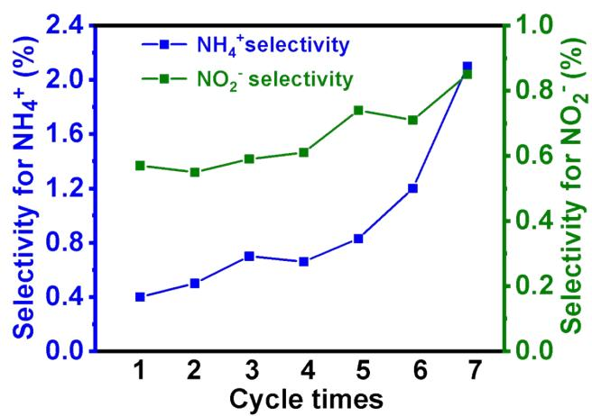
**Fig. S14** nitrite selectivity and ammonia selectivity of Fe/Fe<sub>3</sub>C-NCNF-2 over 7 cycles test of electrocatalytic denitrification. Reaction conditions: initial NO<sub>3</sub><sup>-</sup>-N concentration 100 mg/L, 0.03 M NaCl and 0.01 M Na<sub>2</sub>SO<sub>4</sub>, initial pH value 5 at 24 h.
