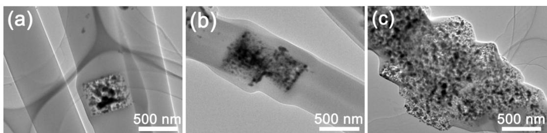
**Fig. S3** (a-c) TEM images of Fe/Fe<sub>3</sub>C-NCNF-1 (iron content: 11%, pyrolysis at 500 °C), Fe/Fe<sub>3</sub>C-NCNF-2 (iron content: 32%, pyrolysis at 500 °C), Fe/Fe<sub>3</sub>C-NCNF-3 (iron content: 41%, pyrolysis at 500 °C).
