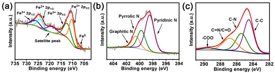
**Fig. S7** High resolution XPS spectra of (a) Fe 2p, (b) N 1s, and (c) C 1s of Fe/Fe<sub>3</sub>C-NCNF-2-400 (iron content: 32%, pyrolysis at 400 °C).
