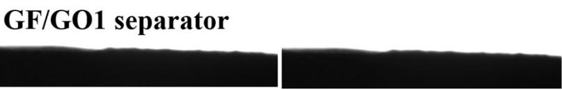
**Fig. S7** Wettability test of GF (a) and GF/GO1 (b) separator.
