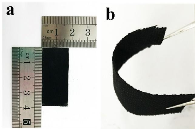
**Fig. S8** Photos of self-supported VS<sub>2</sub>/CC nanoarrays electrodes, which are bent using very small force. This demonstrates the flexibility and light weight of the electrodes.
