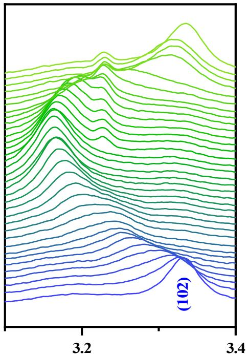
**Fig. S12** In situ XRD profile evolution of diffraction peak 102 of  $\text{VS}_2$  at 0.04C according to the electrochemical discharging and charging profile nearby. It can be seen that after charging the 102 peak restores to the initial position exactly as the other peaks in Fig. 3a and b new diffraction peak appearing during charging does not match with any related substance consisting of V or S, it is most probably coming from the side effects of the electrolytes.
