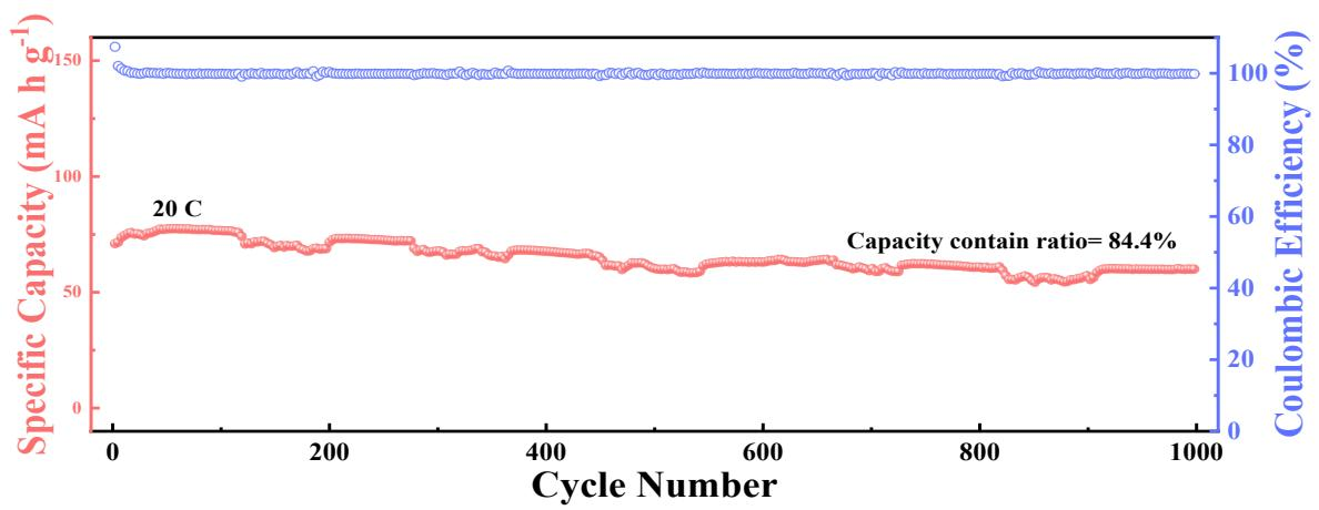
**Fig. S9** Cycle stability test at 20 C for 1000 cycles.
