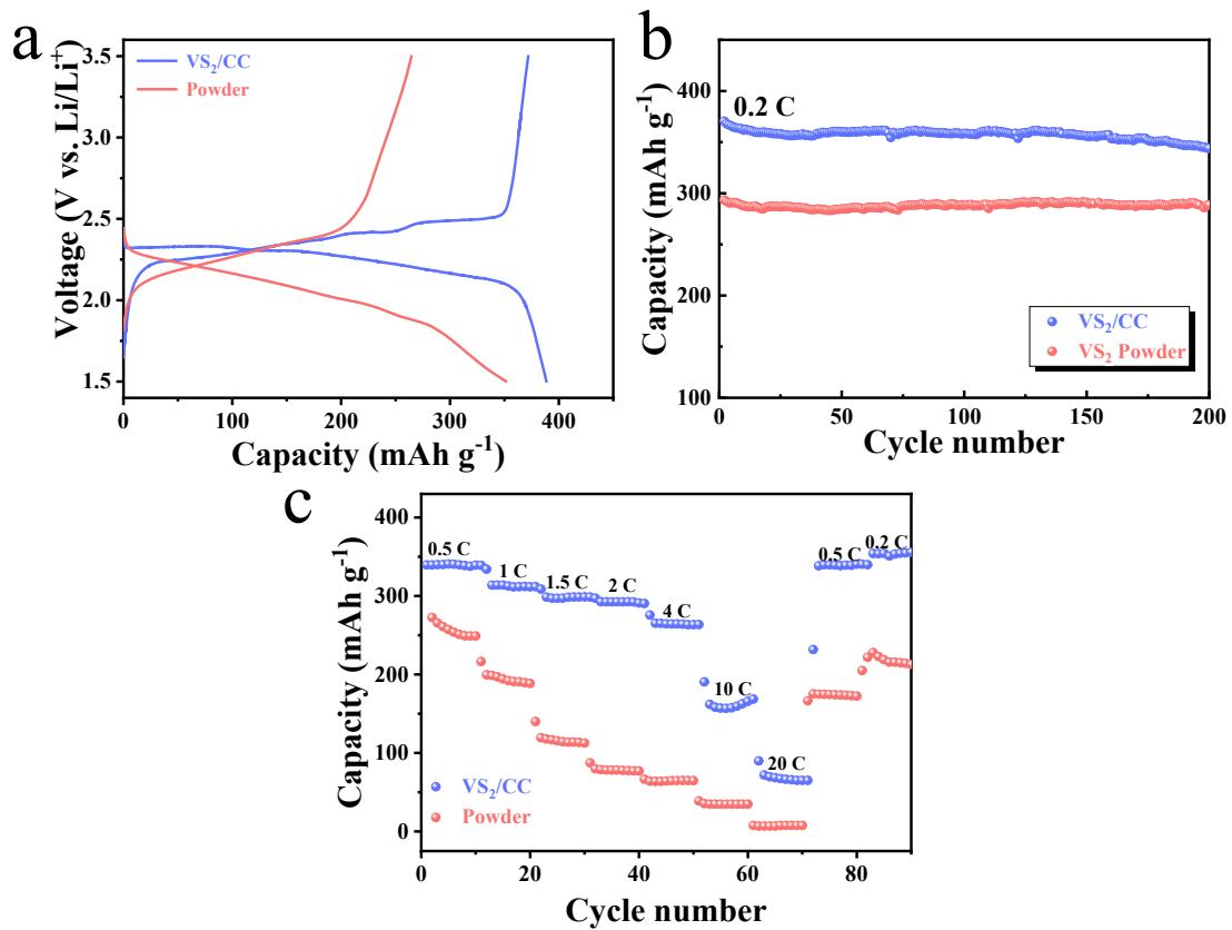
**Fig. S10** a) Charge/discharge curves measured between 1.5 and 3.5 V at a rate of 0.2 C. b) Cycle stability test of VS<sub>2</sub>/CC nanoarrays and VS<sub>2</sub> powder electrodes at 0.2 C for 200 cycle. c) Rate performance of VS<sub>2</sub>/CC nanoarrays electrode and power electrode.
