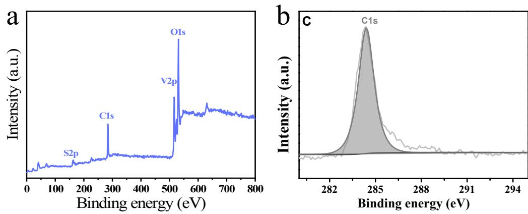
**Fig. S6** XPS spectrum. a) Survey spectra. b) C 1s peaks of VS<sub>2</sub>/CC nanosheet arrays.
