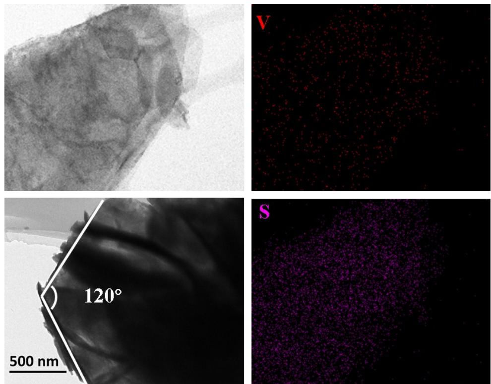
**Fig. S2** TEM images of VS<sub>2</sub> and the corresponding element mapping of V and S.
