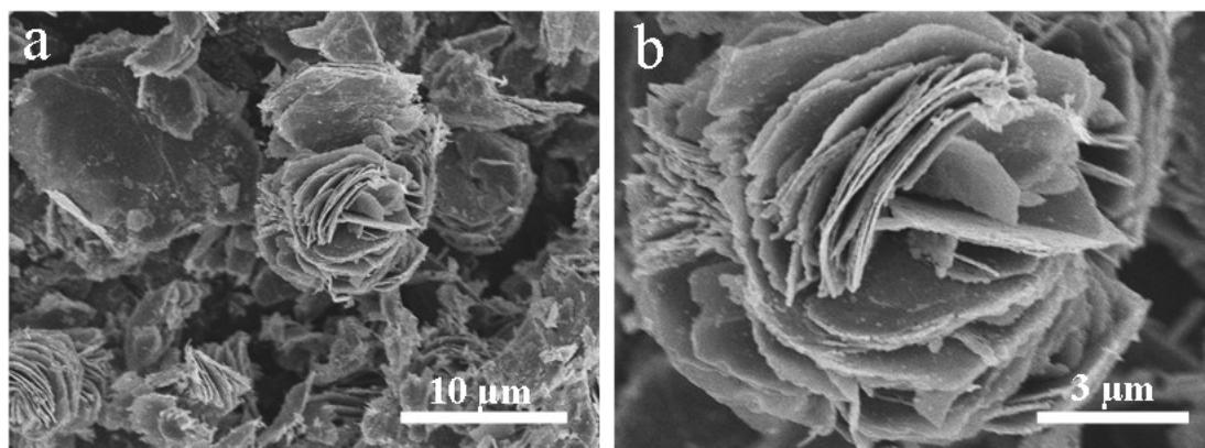
**Fig. S1** SEM images of a) low and b) high magnification of VS<sub>2</sub> powder.
