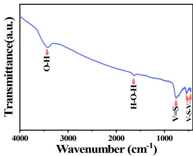
**Fig. S5** The FTIR spectrum of VS<sub>2</sub>/CC nanosheet arrays.
