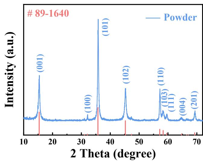
**Fig. S3** XRD patterns of the VS<sub>2</sub> powder.
