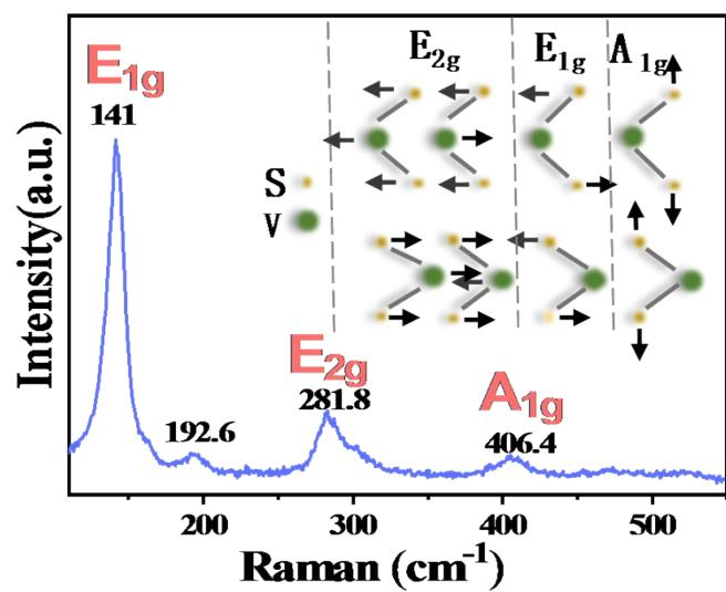
**Fig. S4** The Raman shift spectrum of VS<sub>2</sub>/CC nanosheets arrays.
