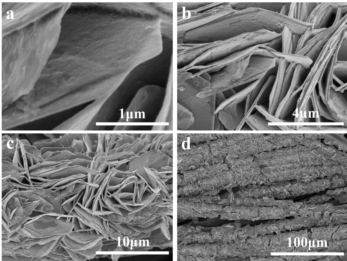
**Fig. S11** SEM images of VS<sub>2</sub>/CC nanoarrays electrode after 200 cycles at different magnification.
