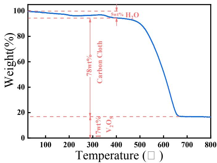
**Fig. S7** TGA curve of VS<sub>2</sub>/CC nanoarrays electrode under an air atmosphere.
